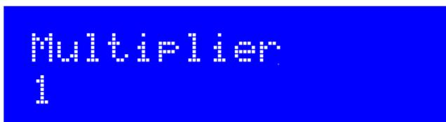
Multiplier allows you to use this signal generator as a VFO in radios where a Quadrature Sampling Detector (for example) is required, that is clocked by a VFO signal at 4x the receive signal. The Clk0 frequency is the displayed frequency + offset, multiplied by the multiplier.
