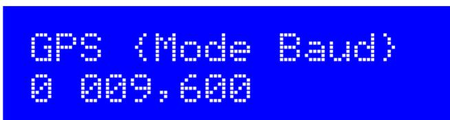
The first setting is the GPS mode. This controls how and whether GPS is used. If set to a non-zero value, and a GPS module is connected and producing a valid 1pps signal, then the accurate time pulses from the GPS unit will be used to discipline the output frequency(s) of the VFO/Signal Generator.
