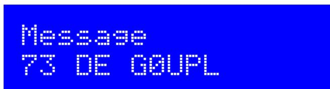
The message setting is an alphanumeric parameter which may be up to 511 characters long. For FSKCW, DFCW, CW, QRSS modes, it must be in the range A – Z, 0 – 9, / or a space character. Hell modes can use punctuation characters as well, but not the \* character.
