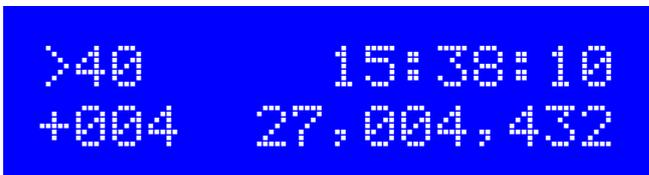
In this example, the calibration just completed has increased the reference clock value by +4Hz to 27,004,432Hz.
