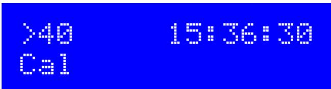
Once the actual frequency calibration starts, the Cal text is followed by a status bar which indicates the progress of the calibration. When calibration has completed, the new reference frequency value for 10 seconds (or whatever Cal Time is set to), as well as the change that was made since the previous calibration. For example:
