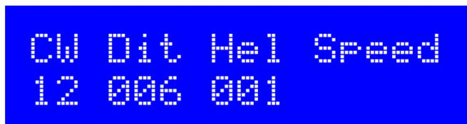
The Speed settings selects the transmission speed for various modes. The default is 00 000 000, at power up.
