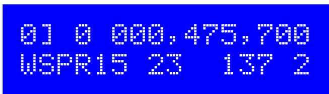
WSPR-15 is a relatively new experimental mode that is a variation of the common WSPR mode. It is used on the LF bands where the higher signal-to-noise ratio it offers is advantageous. WSPR-15 uses the same encoding algorithms as WSPR, but the tone spacing is 8 times closer (approximately 0.18Hz) and the speed is also 8 times slower.
