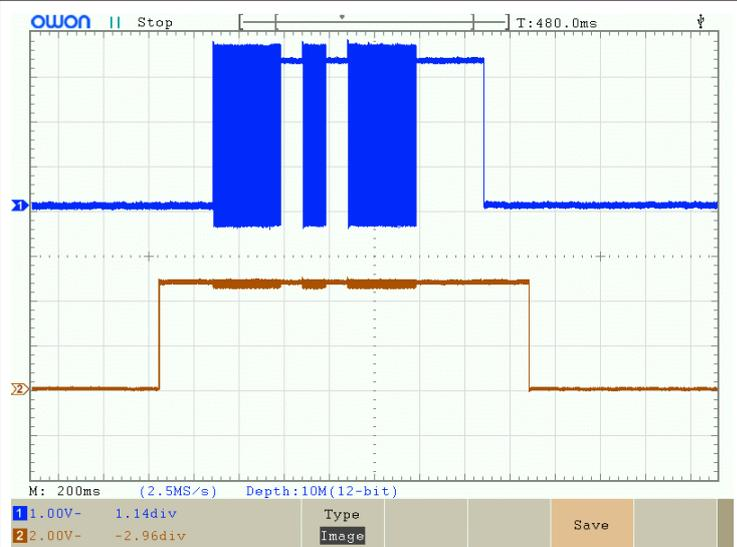
Finally, here the horizontal scale is 1 second per division, and this 'scope trace shows the action of the "PTT" output with the "PTT Delay" parameter set to 550 milliseconds. The moment captured is the gap between two consecutive WSPR transmissions.
