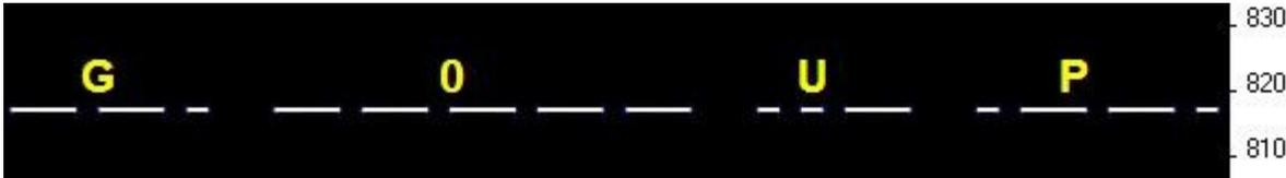
The original plain QRSS mode is simply plain CW, but massively slowed down, typically with dit speeds from 3 seconds or slower, even all the way to 120 seconds in some cases.
