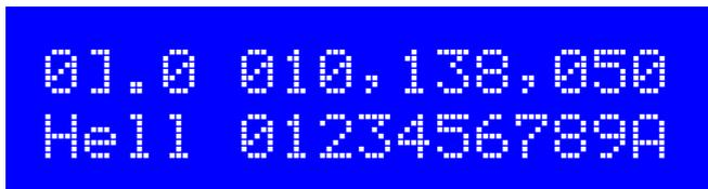
As usual, the display shows the band, mode, frequency and the message scrolls to the left as it is sent.
