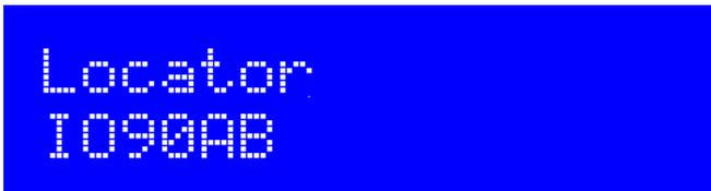
The locator setting is only used in WSPR and PI4 modes, and is one of the inputs to the WSPR encoding algorithm. It is six characters, the first two are always A – R, the second two are numbers in the range 0 – 9, and the final pair are always A – X. Editing this parameter automatically prevents incorrect entries. The locator is not needed for any other mode than WSPR and PI4, and may be left blank if not using these.
