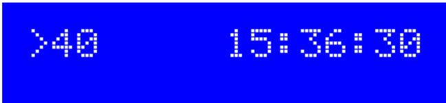
In this example, the time is 15:36:30 and the system is waiting until 40 minutes (time 15:40:00) to start the next message transmission. Additionally the heartbeat will flash, in the space on the top row. When a calibration is about to take place (GPS mode is non-zero) , there will be an additional second line display:
