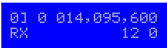
This example illustrates the screen settings that could be used for the reception of 20m WSPR. The reception frequency is the “USB Dial Frequency” listed on the WSPRnet.org website. 14.095600MHz for 20m. This is 1500Hz offset from the centre frequency of the transmitted frequency band.
