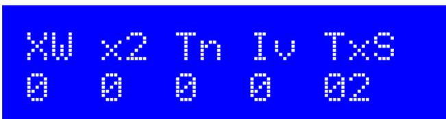
This is a set of configuration parameters that control the Ultimate3S functionality. There are FIVE configuration parameters in one configuration screen; this is to save space and to save time when scrolling through the menu items; since in general these configuration options are not likely to be changed often (if at all). The five settings are described below.
