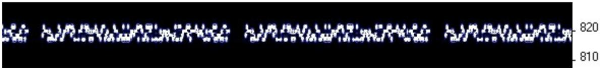
WSPR decoding takes place in the WSPR program by K1JT (see <http://physics.princeton.edu/pulsar/K1JT/wspr.html>). This is a screenshot showing the WSPR 2.0 screen following reception of a few transmissions (output frequency = 1,500Hz, Frame = 02, Start = 00).
