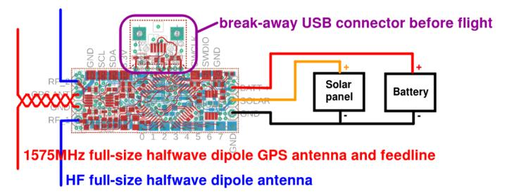
The HF antenna needs 1/4-wavelength on each leg (for example, each leg is 5m for 20m operation). A typical flight configuration has the top end of the top leg tied to the balloon, and the U4B payload suspended directly in the middle of the dipole.
