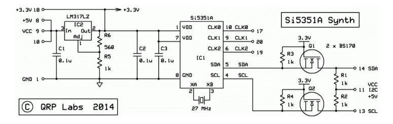
All module pins labeled "GND" are internally connected within the module. Similarly +5V pins (8, 9, 10) are also internally connected on the module PCB. Pin 11 is the pull-up resistor positive supply voltage for the level converters. For ordinary use, with a +5V I2C bus, pin 11 should be connected to +5V. The connection is provided separately (not connected to +5V internally) in case you wish to use a different I2C bus voltage.
