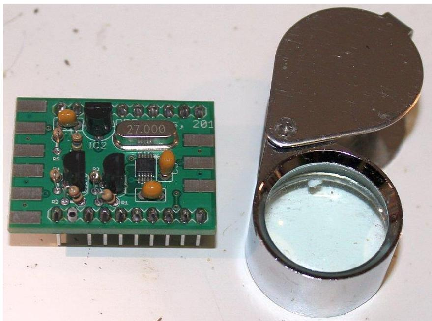
Check the resistors are installed in the right place (remember R6 is 560 ohms) and the voltage regulator is IC2 (don't mix LM317LZ and BS170!). Check the Si5351A chip is nicely soldered too: even factory SMD robots might make mistakes sometimes!
