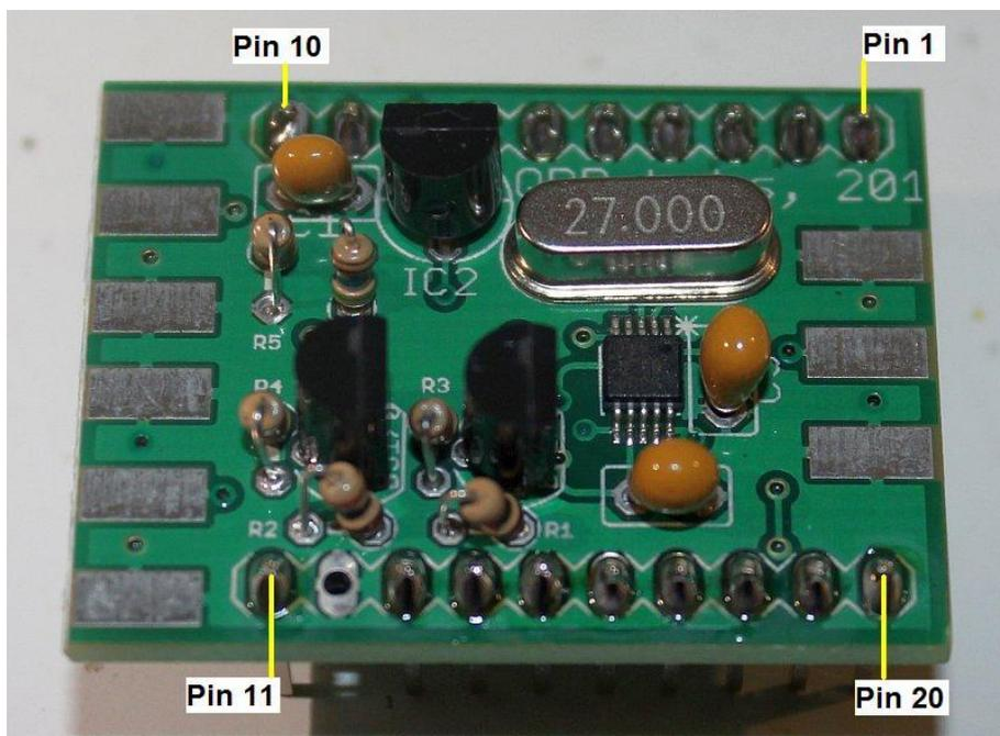
Note that in relating the pinout to the physical module, designated pin 1 is near the shorter PCB end of the module, as shown in this photograph. The photograph is an earlier PCB revision without the TXCO pad.
