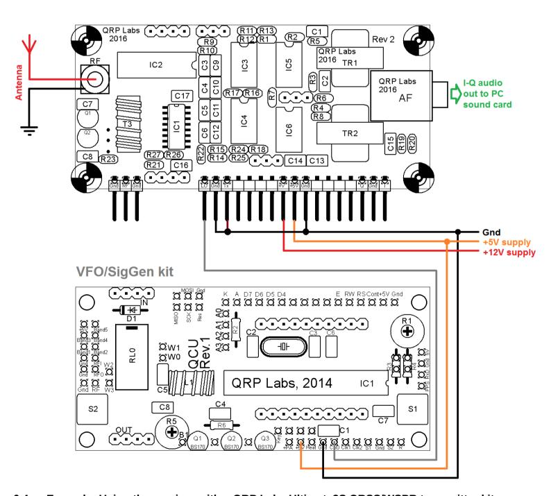
6.4 Example: Using the receiver with a QRP Labs Ultimate3S QRSS/WSPR transmitter kit
