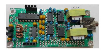
You can test that the wires are properly soldered, as follows. First check for continuity between the RF input and ground. This tests the first winding. The easiest way to do this is just at the "RF" and adjacent "Gnd" pads at the board edge. Hold the black and red probes on the pads as indicated.
