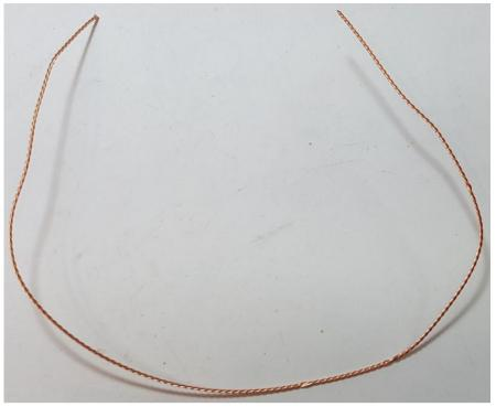
Now cut off the untidy ends, and this is the piece of wire that will be used to wind the FT37-43 toroidal core as a trifilar transformer.
