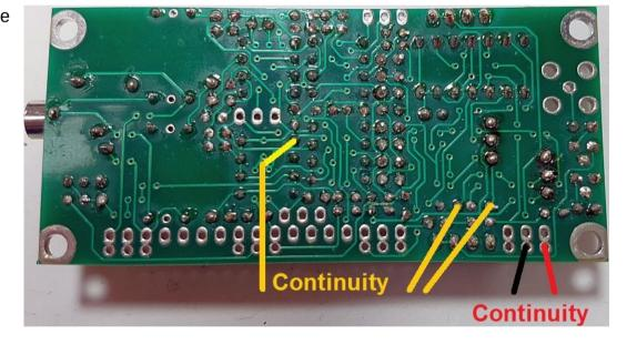
resistors R26 and R27. Hold the black probe on IC6 pin 1. Hold the red probe on the resistor ends as indicated by the two nearby orange lines.
