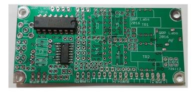
opposite diagonal ends of the chip. Then you can check that the chip is nicely seated on the board before soldering all the other pins. It is easy to make adjustments when only two pins are soldered, by re-heating the joints. But you cannot do that when you have 16 pins soldered! When you're happy with the position of the IC, solder all the other pins.
