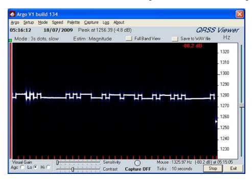
The "gimmick" capacitor C3 will need to be adjusted, to bring the "height" of the FSK to around 4-5Hz. Do not waste spectrum by using more! Less may be sufficient and preferable! Twist C3 tighter to increase the shift, or unwind/snip some wire to decrease it.
