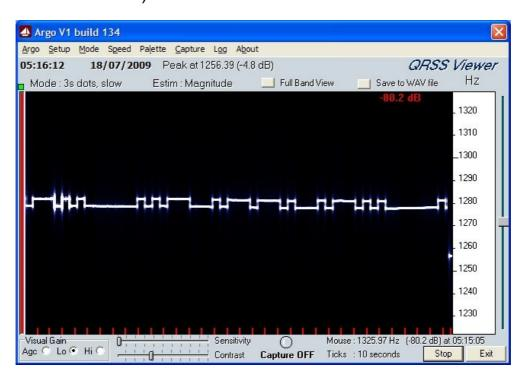
The "height" of the FSK should be around 4-5Hz, and you can adjust this from the Arduino sketch. If the height remains too large, you can cut a piece off the "gimmick" capacitor C3. Do not waste spectrum by using more! Less may be sufficient and preferable!
