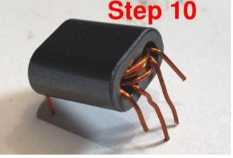
The transformer is now ready for installation in the PCB!
