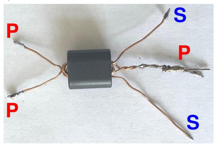
Now re-test with the DVM – points P (P is for primary) should all show continuity to each other; there should be continuity between points S (S is for secondary). But there must be NO continuity between P and S! If there is: you made a mistake, or you have copper wire shorts somewhere.
