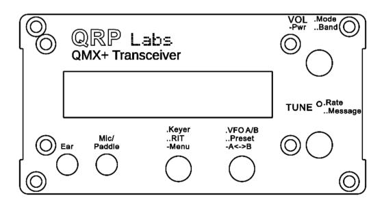
This is the front panel of the QMX+. The Earphone and Mic/Paddle 3.5mm connectors are on the FRONT panel of the QMX+. The pinouts are the same as for the QMX (described above).
