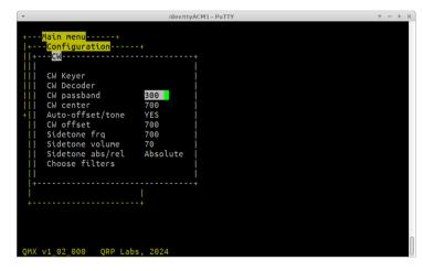
Selects the CW passband. The available options are None, 50, 100, 150, 200, 250, 300, 400 and 500 (Hz). The "None" option disables the CW filter completely and the audio filter remains the default 150-3200Hz wide filter used for Digital modes.
