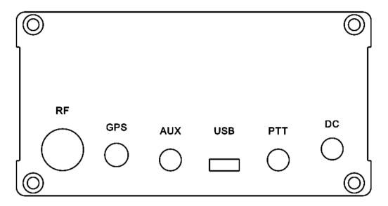
This is the rear panel of QMX+. The RF, USB, PTT and DC connectors are exactly the same as described in the section above. The Paddle/Mic and Earphones connectors are on the QMX+ front panel (see below).
