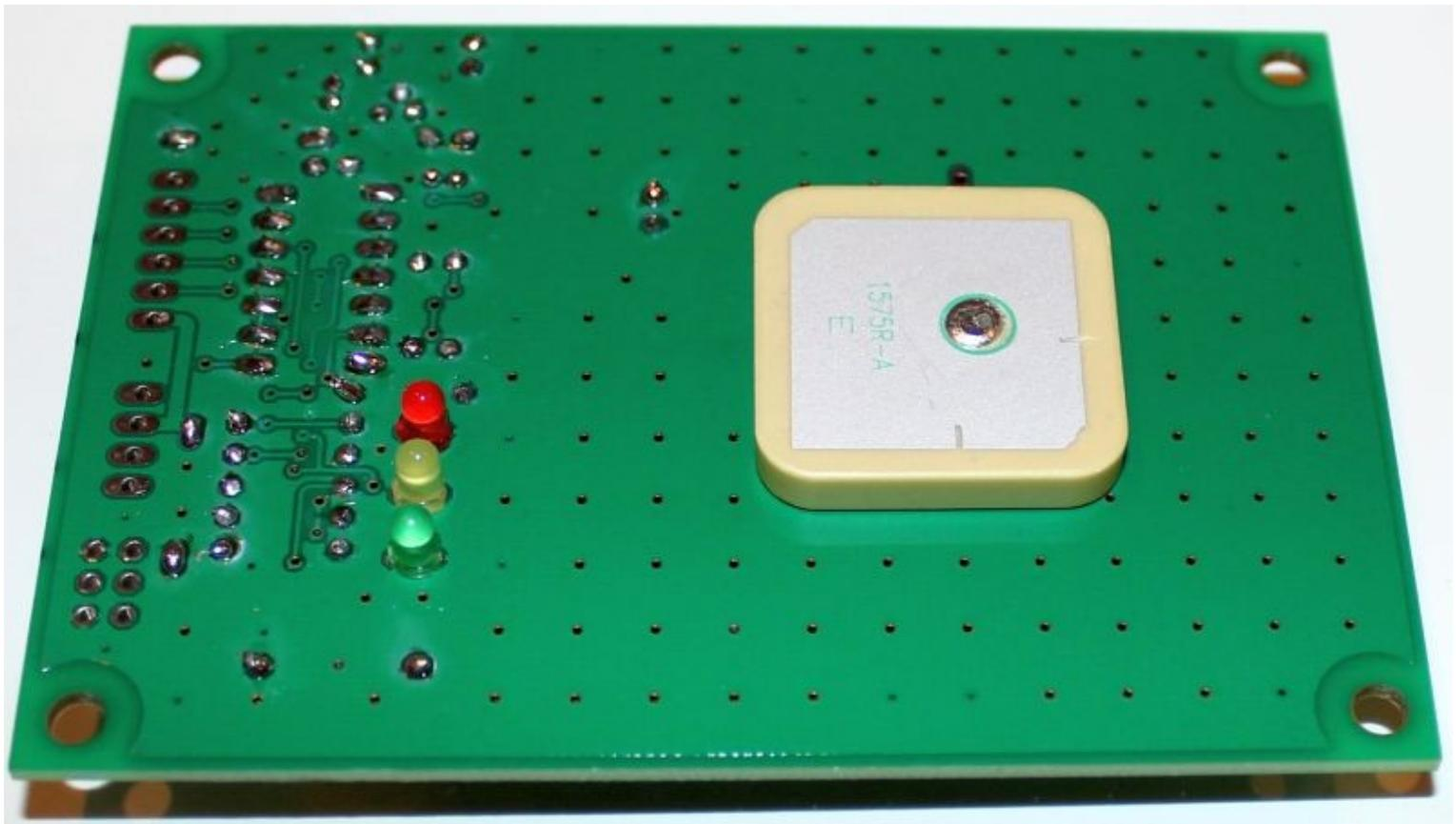
The patch antenna connection pin is not in the exact centre of the square patch. Please refer to the photograph (above). The connection pin should be furthest away from the through-hole components section of the PCB, as shown. The patch should be positioned on the solder side of the PCB.
