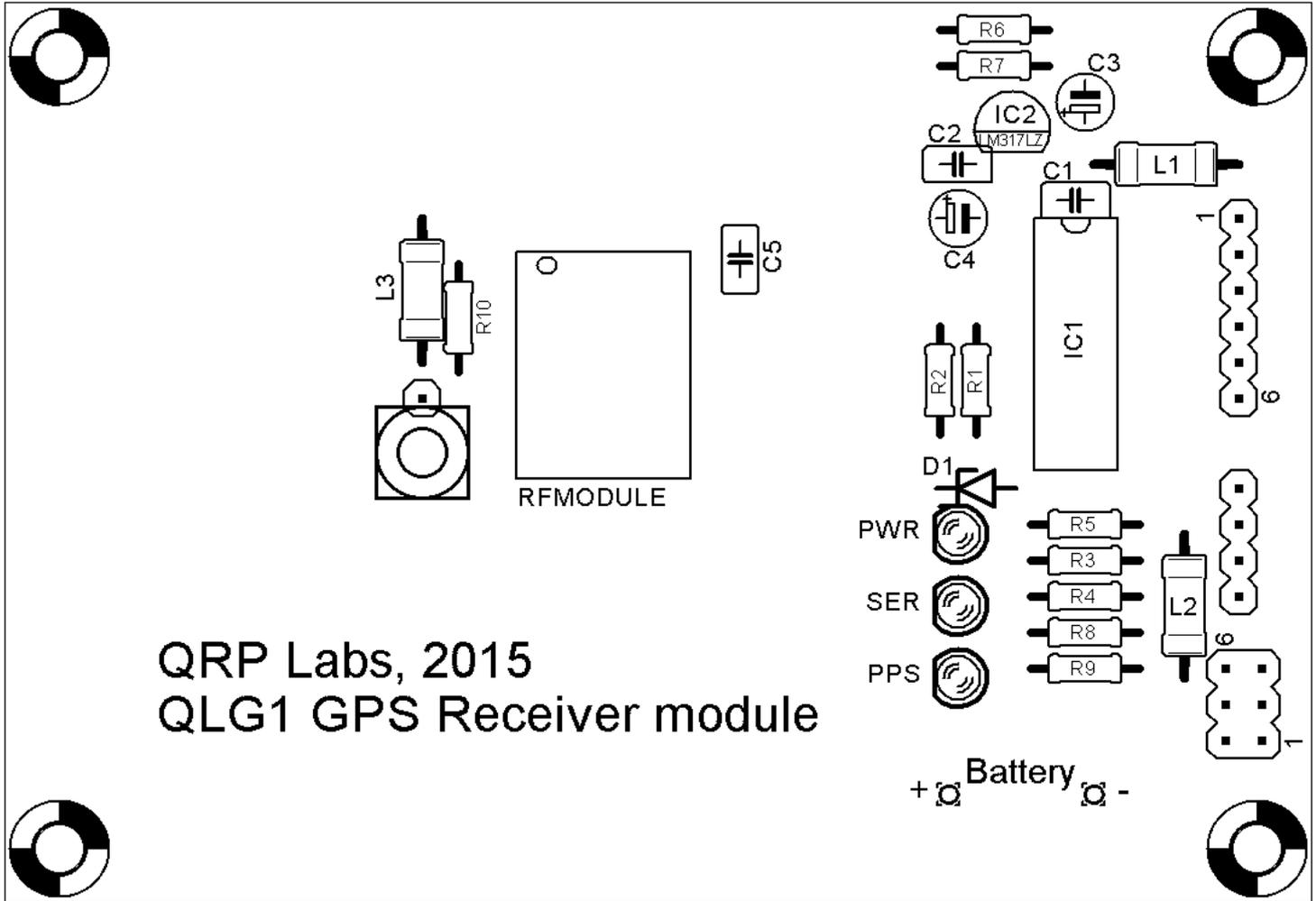
Pay special attention to the orientation of the semiconductor IC1. The dimple in the PCB silkscreen must be aligned with the dimple at the top of IC1.
