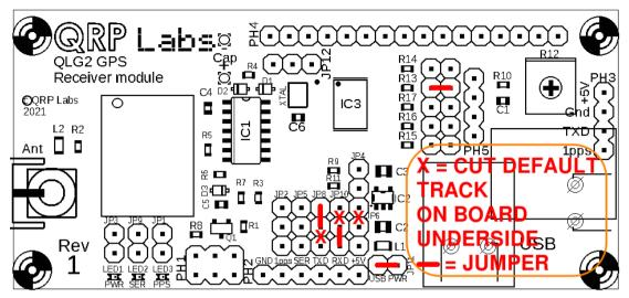
Connection of serial ports 1 and 2 (and also 3 if you have a pre-Rev 3 PCB) requires soldering wires directly to the microcontroller pins, a task to be undertaken with considerable care, to say the least. The Rev 5 PCB has pin headers at the board edge for most of these connections and is very easy.
