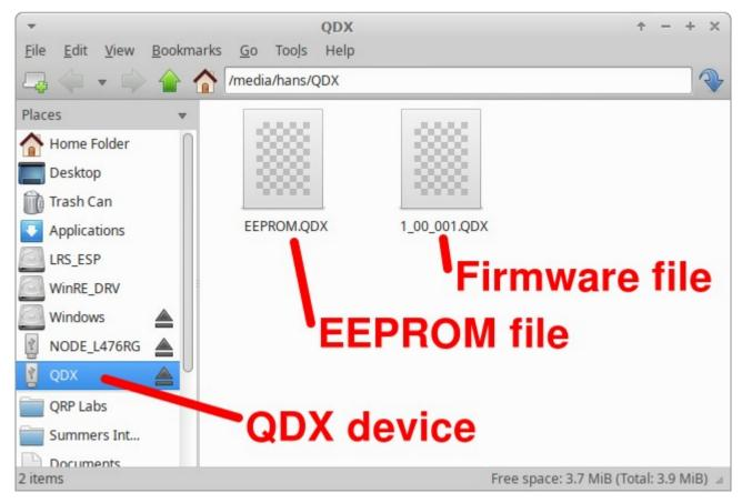
QDX appears as a removable USB Flash device named "QDX", and the folder two files. The firmware file in this example is named shows a single file which is the firmware version file, 1\_00\_001.QDX in this example. The EEPROM file is always named EEPROM.QDX. You can read and write EEPROM files in order to make and restore backup copies of your configuration etc.
