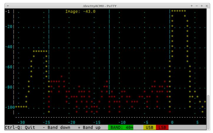
Configuration screen, then sweeps the signal generator input from -30.5kHz (below) to +7kHz (above). An example of the resulting sweep is shown below:
