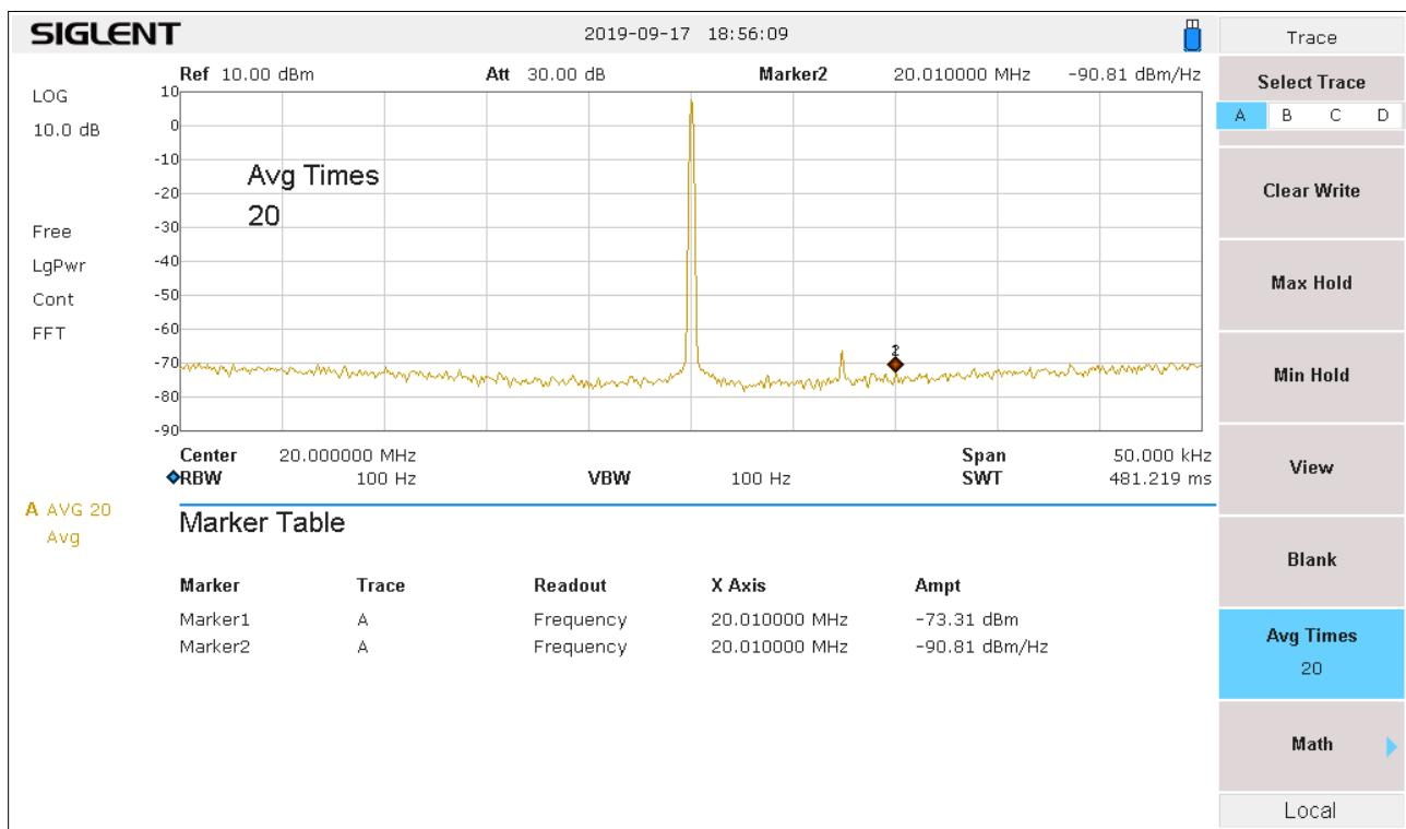
In the example below. You were running I think -7.5 dBm out of your filter into your operational RF amp which has +19 dB gain. So your carrier reference seen on your screen would be around +11.5 dBm (-7.5 +19)
