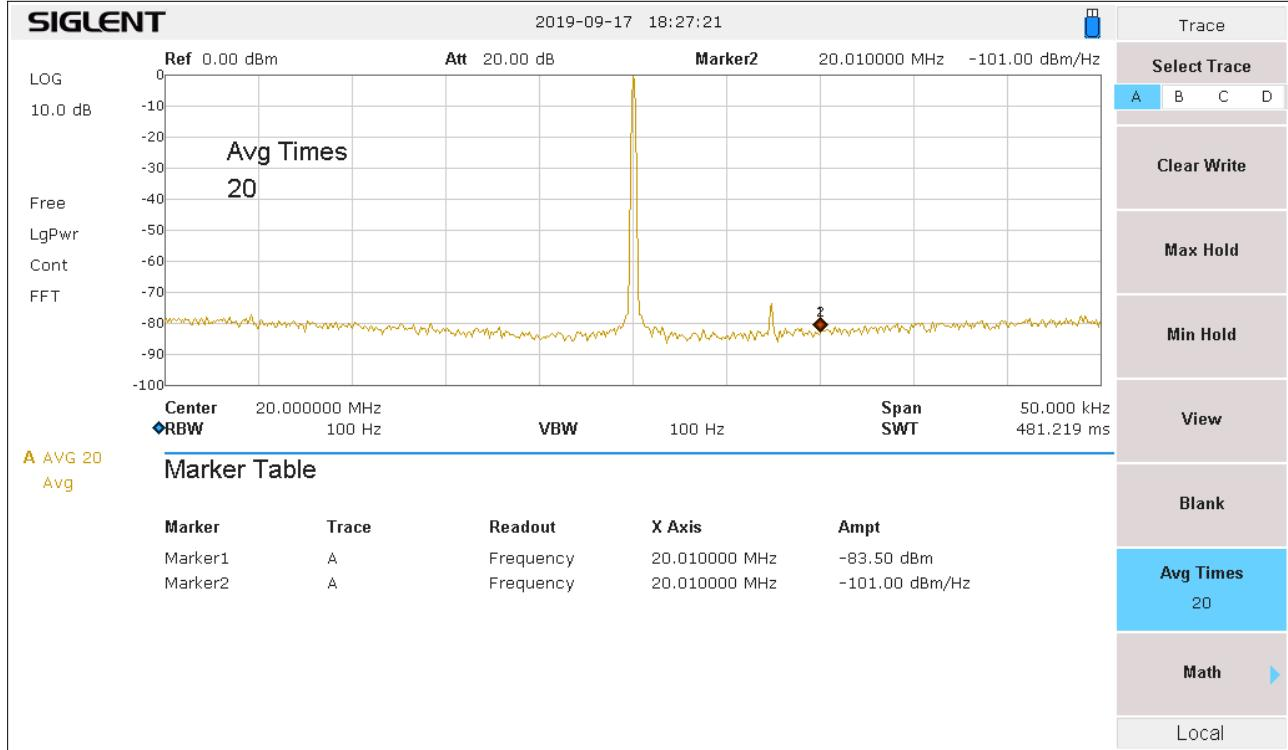
The plot is taken with 100 Hz Resolution bandwidth and 100Hz video bandwidth, but with 20 trace averages. One can see the noise is fractionally quieter (0.9 dB), probably closer due to multiple averages, whereas the 1Hz video B/w sweep is the result of one sweep
