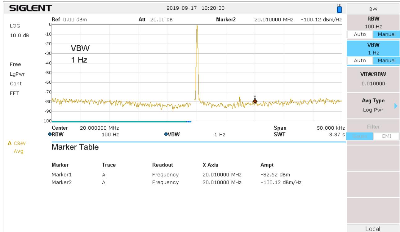
The plot is taken with 100 Hz Resolution bandwidth and 1Hz video bandwidth,
