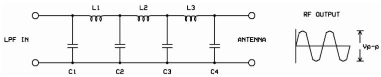
The design uses four capacitors and three inductors wound on toroids, and has 50-ohm input and output impedance. The small PCB has a 4-pin plug at its input and output. It is designed to fit onto the "Ultimate2" multi-mode QRSS/WSPR transmitter kit, but may of course be used as a LPF for other QRP transmitter designs. It also fits the relay-switched LPF kit.
