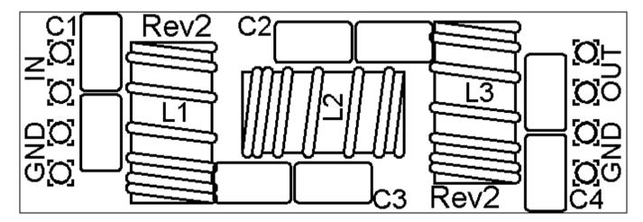
The PCB is quite small and the parts are close together. You are recommended to use a low wattage iron with a fine tip, and fine solder e.g. 1mm diameter or less. Take care not to overheat the PCB and risk damaging it. A well-lit area and magnifying glass may assist. Be careful not to bridge solder across closely-packed connections. I recommend checking with a DVM to make sure no solder bridges have been inadvertently created. Take care to ensure correct alignment of the 4-pin plugs.
