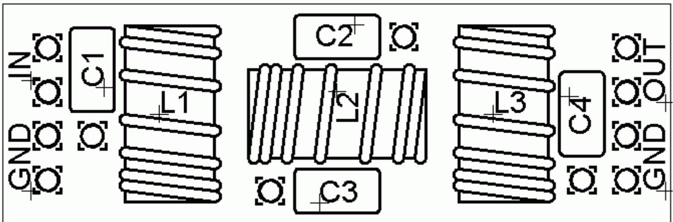
The PCB is quite small and the parts are close together. You are recommended to use a low wattage iron with a fine tip, and fine solder e.g. 1mm diameter or less. Take care not to overheat the PCB and risk damaging it. A well-lit area and magnifying glass can assist. Be careful not to bridge solder across closely-packed connections. I recommend checking with a DVM to make sure no solder bridges have been inadvertently created. Take care to ensure correct alignment of the 4-pin plugs.
