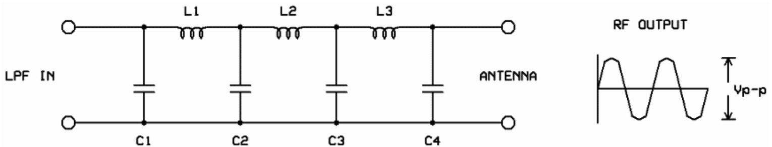
The design uses four capacitors and three inductors wound on micrometals toroids and has 50-ohm input and output impedance. The small PCB has a 4-pin plug at its input and output. It is designed to fit onto the "Ultimate2" multi-mode QRSS/WSPR transmitter kit, but may of course be used as a LPF for other QRP transmitter designs.
