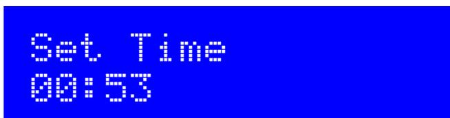
This setting is only required if you have NOT connected a GPS receiver module to the kit. If a GPS is connected, the time should be set automatically.
