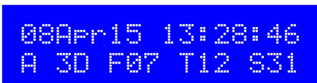
The display shows date and time on the top line, followed by GPS satellite reception information on the bottom line. The heartbeat will blink in the space between the date and time on the top line.
