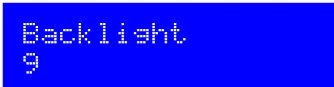
This setting allows the LCD screen's blue LED backlight brightness to be adjusted. The default value is 9 (maximum brightness). 0 corresponds to minimum brightness – the backlight is switched off.
