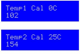
These are the calibration values for the temperature sensor when the temperature is 0 and 25 centigrade. The system assumes a linear relationship between the voltage from the temperature sensor, and temperature. In order to calibrate the temperature, two settings are required, at 0C and 25C.
