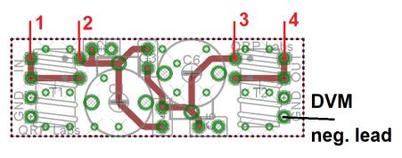
on one of the ground pins, and hold the positive probe to each of the points labelled 1-4 in this diagram. You should measure 0 ohms in every case! If you do not – then it means you have either connected something wrongly, or have not properly scraped/burnt off the enamel wire insulation! So go back and check everything!
