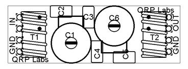
respectively. Do NOT solder the winding ends into the PCB pad holes yet! It is very difficult to remove and adjust the number of wire turns, once the wire end is soldered in place!
