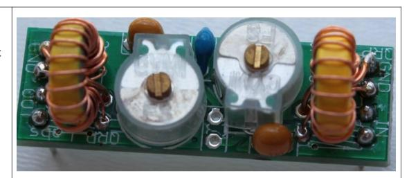
Maximum capacitance ("closed"). You can see that the plates of the trimmer capacitors overlap each other completely.
