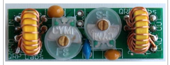
Half-way state – the plates of the capacitors half overlap.
