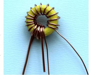
Below left: the completed pair of 15m band toroidal
