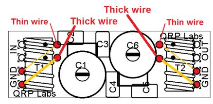
(for T2). The other ends of the toroidal transformer windings are both connected to ground pins ("GND") so it does not matter which is the thin wire and which is the thick wire.
