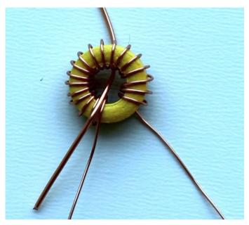
The photo (right) shows the completed second winding (thick wire). There are THREE turns in the 15m BPF. Check the number of turns required, for the band you are building (see parts list). Remember
