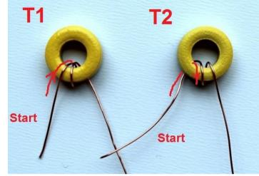
This diagram (right) shows where the toroid wires will be soldered. The yellow coloured lines indicate the toroid windings.
