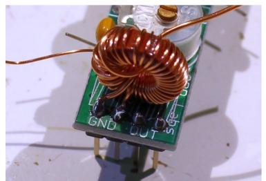
to the header pin – this could melt the black header plastic on the other side of the PCB. Instead, hold the
