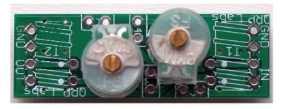
When soldering the pins, try to be FAST. You don't want to risk melting the plastic of the capacitor insulation and body.
