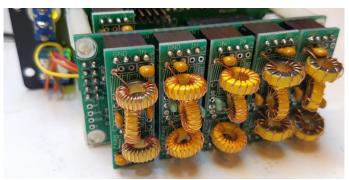
The 60m band LPF filter is plugged into the socket on the main VFO/SigGen board; the other LPFs 40, 30, 20, 15 and 10m are plugged into the relay board. The display is configured simply
