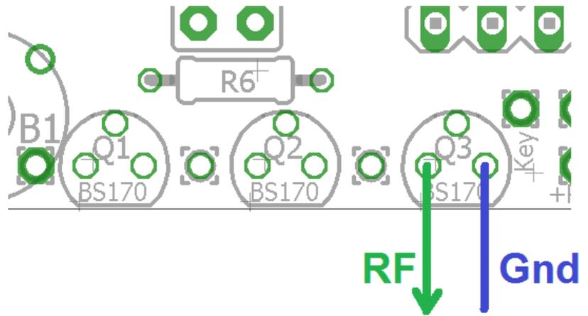
When connecting the RF output of the 5W HF PA back to the filter input on the Ultimate3S, it is convenient to use the pins of the 2 x 5 header as shown. The RF output on the HF PA PCB is
