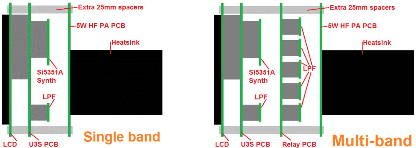
Please refer to section 5.4 of the PA kit assembly manual “Heatsink temperature rise; PA kit installation in enclosure” to decide how to enclose the system – it may require additional heatsinking or fan-assisted cooling.
