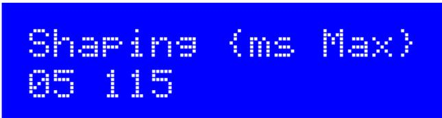
The first parameter is the rise/fall time of the raised cosine envelope that will be generated. In this example it is 5ms. Rise/fall times of around 5 to 10ms are common in commercial amateur radio CW transceivers.
