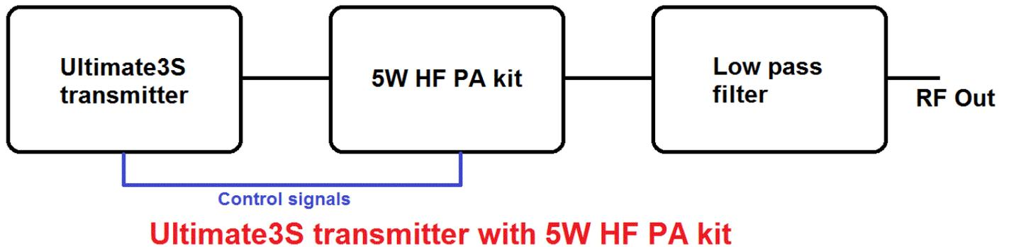
The basic Ultimate3S transmitter is shown in the top half of this diagram. The Low Pass Filter (the LPF) is drawn as a separate block to the Ultimate3S transmitter. In reality the LPF is a plug-in module on the Ultimate3S PCB. If you are running a multi-band Ultimate3S then there is a LPF plugged into your Ultimate3S PCB, and a 5-band Relay-switched extension PCB bolted behind that. As far as the 5W HF PA kit is concerned, the principles are the same in the single-band and multi-band cases.
