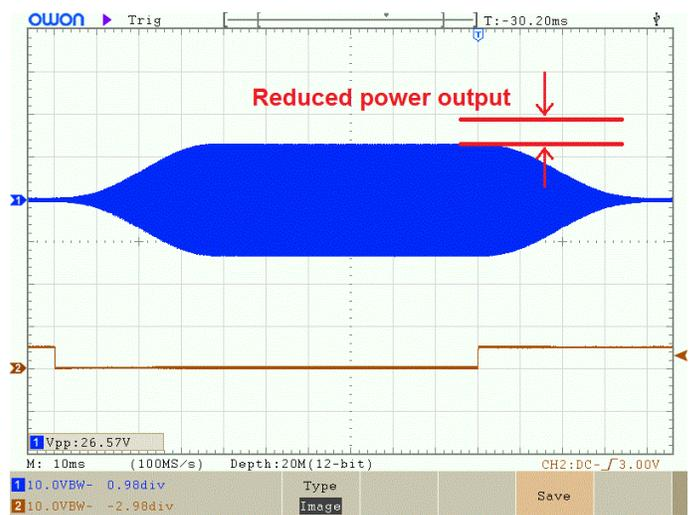
If the "Max" value is too high (above left), then there will be clipping (a sharp corner) at the start and finish of the transmission, and there will be a delay from key-up to the decline of the RF envelope. On the other hand if the "Max" value is too low (above right) then the envelope will have a nice raised cosine shape but will have a reduced amplitude (power output).
