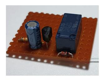
The resistor and capacitor in the base circuit of the transistor form an integrator which ignores the rapid pulses of the LCD write. It also delays the activation of the relay activation/de-activation. But this will usually not be critical. The "Aux" parameter is effected on the LCD signals D4-D7 at the end of the prior transmission. So in the case of a sequence of WSPR transmissions for example, the next Aux
