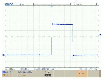
kit writes the current symbol transmitted to the display on the bottom row. Again the trace shows the D7 output and D7 is configured to be zero (low). Note the short burst of activity on the D7 signal, which occurs once per WSPR symbol (every 0.68 seconds).
