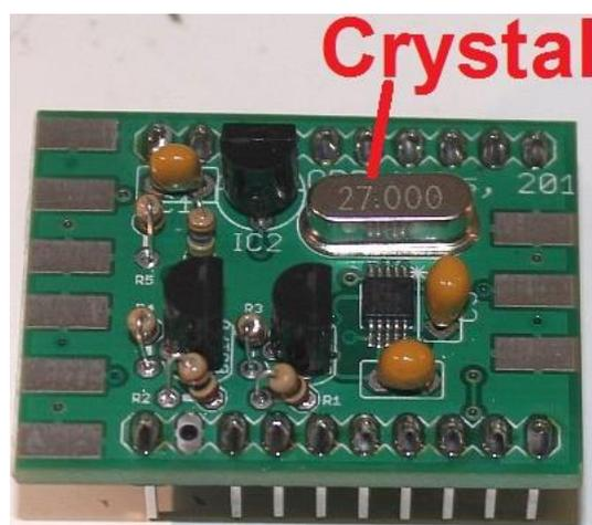
sensitivity. In fact this is not the case. The oscillator is made up of both the resonant component (the quartz crystal), and active amplification and biasing components within the Si5351A chip itself. These internal components also have temperature sensitivity and can alter the oscillator frequency. Therefore improving drift requires consideration of all these sources of drift.
