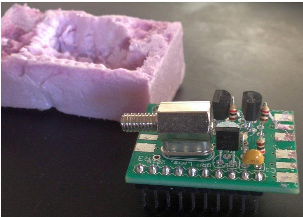
Jon Ove carved out a piece of foam to fit over the top of the Si5351A board. But good results can even be obtained simply by installing the Ultimate3S unto an enclosure such as the standard QRP Labs enclosure. That is sufficient to keep air currents away and greatly reduces the drift. But for sure, Jon Ove's solution is more thorough and elegant.
