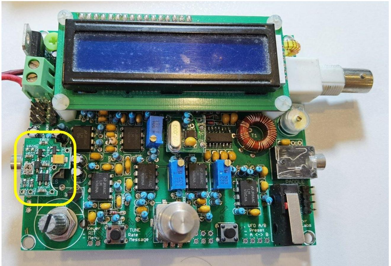
Before gluing it down, solder on five hookup wires for the five connections.
