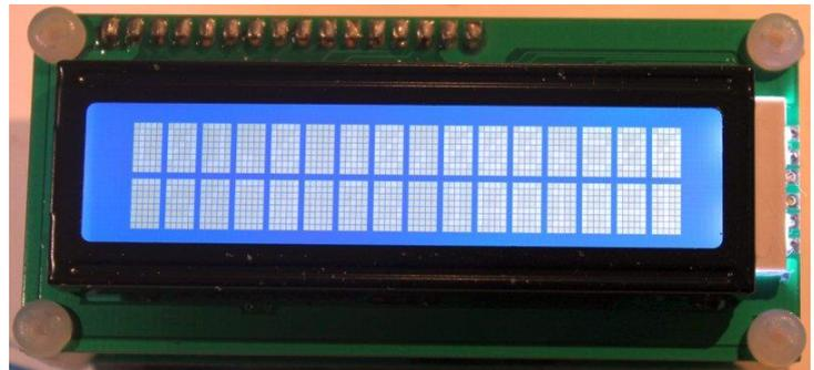
When you see "Diagnostic Mode" it means all is well with the processor and the LCD communication. When you press the left button, diagnostic mode will be cleared. Then you should see the splash screen, which shows the firmware type and version number.
