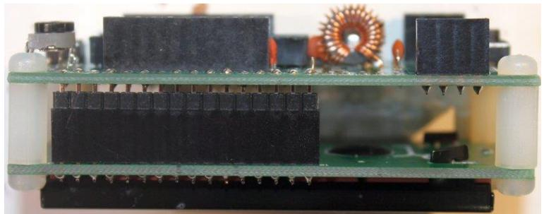
The combined 16-way plug and socket when mated together, have a height of a little under 12mm. Therefore it is necessary to have a gap somewhere.
