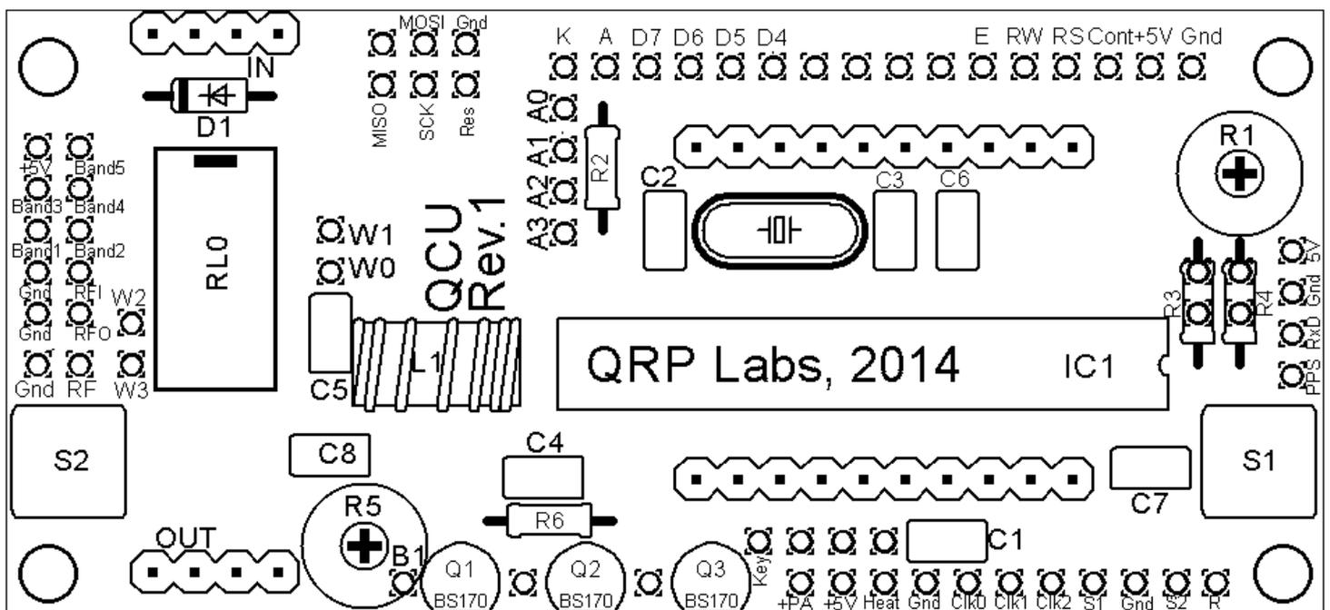
Pay special attention to the orientation of the semiconductors. For IC1, the dimple in the PCB silkscreen must be aligned with the dimple at the top of the IC socket and the IC.
