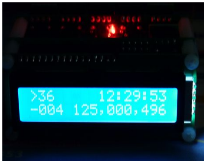
The Test U3 with 28MHz WSPR transmission from the signal source U3. The Test U3 has just completed a successful calibration during the WSPR.
