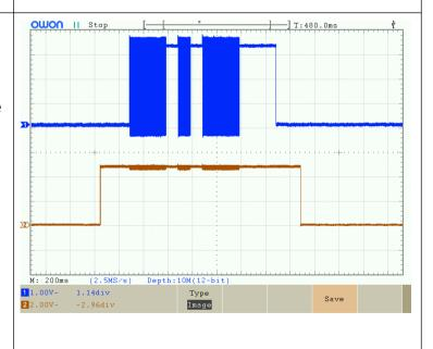
Finally, here the horizontal scale is 1 second per division, and this 'scope trace shows the action of the "PTT" output with the "PTT Delay" parameter set to 550 milliseconds. The moment captured is the gap between two consecutive WSPR transmissions.
