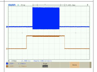
This is the CW "K" at 12wpm, now with the "PTT Delay" parameter is set to 200 milliseconds. Note that the entire message being sent is just a single "K" for illustrative purposes.
