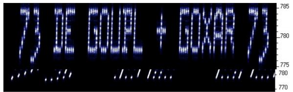
The following image shows part of the same thing in Argo's 3 second "slow" mode. The larger fourier transform bucket size means the image is more clear, but the faster scroll rate makes the letter's height to width ratio somewhat less attractive. Other slow-speed fourier transform software present more configuration options and may be more suited for slow-Hellshreiber reception than Argo.
