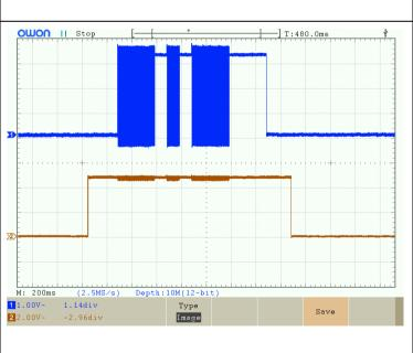
Finally, here the horizontal scale is 1 second per division, and this 'scope trace shows the action of the "PTT" output with the "PTT Delay" parameter set to 550 milliseconds. The moment captured is the gap between two consecutive WSPR transmissions.
