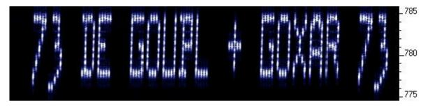
The following image shows part of the same thing in Argo's 3 second "slow" mode. The larger fourier transform bucket size means the image is more clear, but the faster scroll rate makes the letter's height to width ratio somewhat less attractive. Other slow-speed fourier transform software present more configuration options and may be more suited for slow-Hellshreiber reception than Argo.
