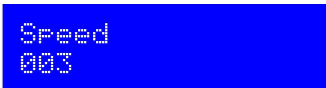
The Speed setting selects the dit speed, in seconds, for the following modes: FSKCW, QRSS, DFCW. In CW and FSK modes, the Speed setting means Words Per Minute. In Slow-Hell mode, the setting is the number of seconds duration of one character (see later section for explanation). The setting has no effect at all, in CW ID, Hell, DX Hell, WSPR or WSPR-15 modes; these modes all have a defined timing which cannot be changed. It also has no effect in the TX mode.
