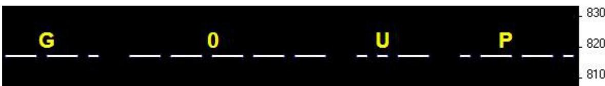
The original plain QRSS mode is simply plain CW, but massively slowed down, typically with dit speeds from 3 seconds or slower, even all the way to 120 seconds in some cases.
