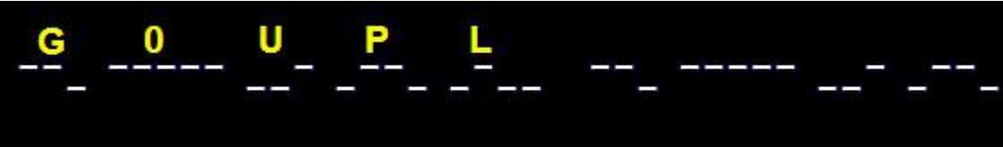
DFCW means dual-frequency CW. The dits and dahs are the same length, but dahs are shifted upwards by the FSK amount. A 1/3 dit-length gap inserted between symbols improves the readability.
