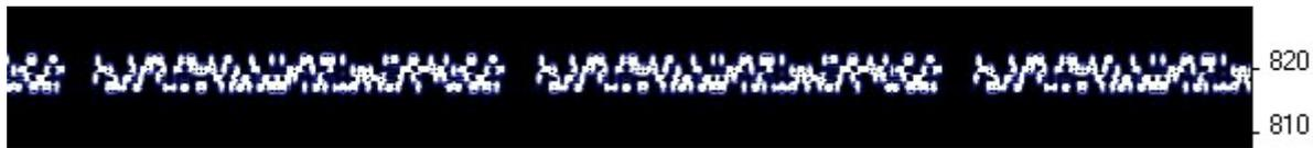
WSPR decoding takes place in the WSPR program by K1JT (see <http://physics.princeton.edu/pulsar/K1JT/wspr.html>). This is a screenshot showing the WSPR 2.0 screen following reception of a few transmissions (output frequency = 1,500Hz, Frame = 02, Start = 00).
