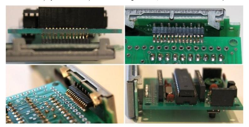
Step 1: Insert the LCD from the bottom of the board. I suggest soldering just the two end pins only, and solder from the top side of the board: this allows un-soldering easily in the event tat However, leave a gap of a few mm, as seen in the top left photo above. That is very important! It allows space for bending the pins at right-angles.
