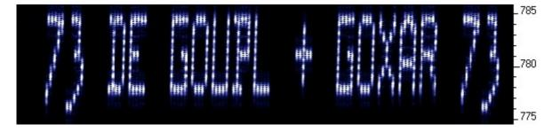
The following image shows part of the same thing in Argo's 3 second "slow" mode. The larger fourier transform bucket size means the image is more clear, but the faster scroll rate makes the letter's height to width ratio somewhat less attractive. Other slow-speed fourier transform software present more configuration options and may be more suited for slow-Hellshreiber reception than Argo.
