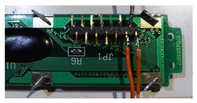
Method 2: LCD mounted directly to the reverse of the board
