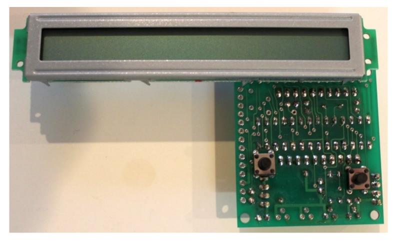
This method is probably the easiest and most direct. The LCD is just soldered in position on the reverse of the board. Make the solder joints on the component side of the PCB. The two buttons are in this case directly accessible. The disadvantage is that the board components are now upside-down! In this configuration you might want to mount some 40mm long bolts in the main PCB corner holes, in order to lift the PCB up, as if on pillars, so that it is not resting on the components underneath.
