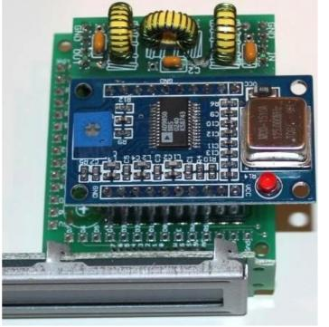
cycle of the DDS square wave. You should not need to adjust this potentiometer, as I have already adjusted it individually, when I tested every DDS module before putting it in a kit. However, some builders have noted that the potentiometer needs to be adjusted slightly for best output waveform on 10m (28MHz). The adjustments needed are extremely slight, the potentiometer setting is very sensitive.
