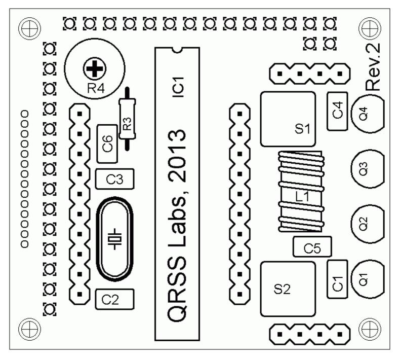
Pay special attention to the orientation of the semiconductors. For IC1, the dimple in the PCB silkscreen must be aligned with the dimple at the top of the IC socket and the IC.
