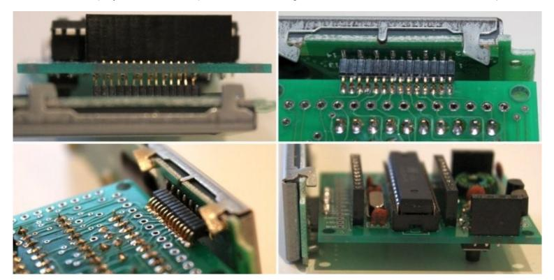
Step 1: Insert the LCD from the bottom of the board. I suggest soldering just the two end pins only, and solder from the top side of the board: this allows un-soldering easily in the event tat However, leave a gap of a few mm, as seen in the top left photo above. That is very important! It allows space for bending the pins at right-angles.
