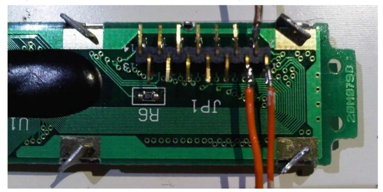
Method 2: LCD mounted directly to the reverse of the board
