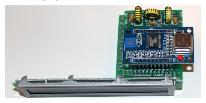
This method is really my favourite method, because it allows the LCD to face the front, convenient for mounting in a front panel.
