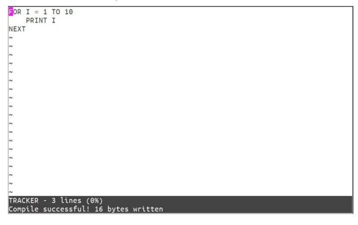
Now pressing Ctrl-C compiles the file, and writes it to disk as a Compiled file. If there are any errors, the compilation will fail without writing to disk, and the error will be identified on the bottom line. Note that the size of the compiled file is generally significantly less than when it was a text file.
