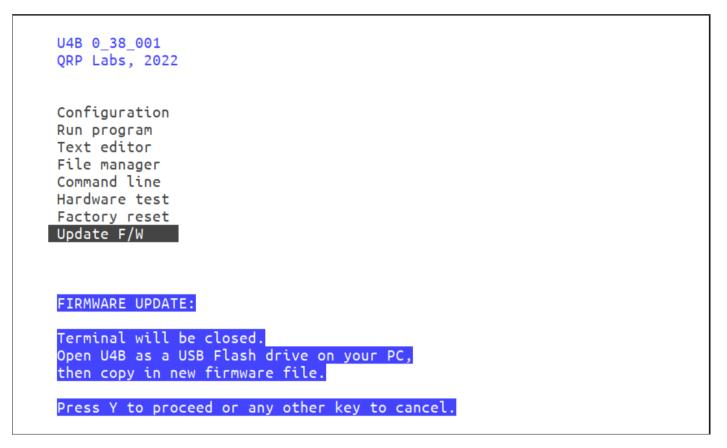
Selecting firmware update, then pressing the Y key proceeds with putting the U4B into bootloader mode. You must then remove the power, and re-apply power; when power is applied in bootloader mode, the U4B onboard LED will flash steadily.
