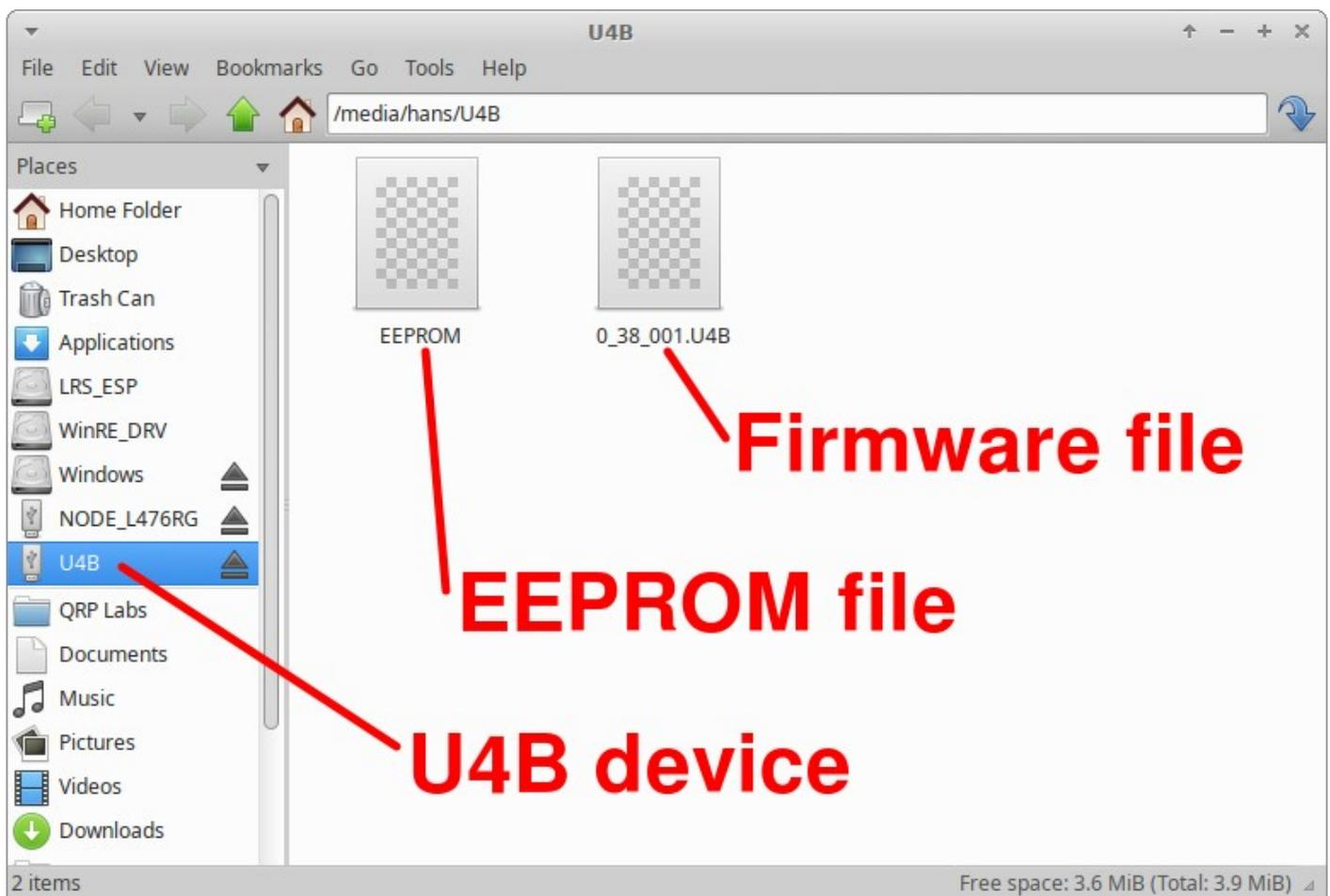
U4B appears as a removable USB Flash device named “U4B”, and the folder contains two files. The firmware file shows as a single file which in this example is named 0\_38\_001.U4B. The EEPROM file is always named EEPROM. You can read and write EEPROM files in order to make and restore backup copies of your configuration etc.
