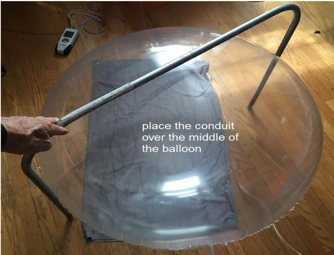
Put the measurement gizmo in place in the middle of the conduit till the bottom of the gizmo touches the top of the balloon and slide down the paper slider till it touches the upper side of the conduit.
