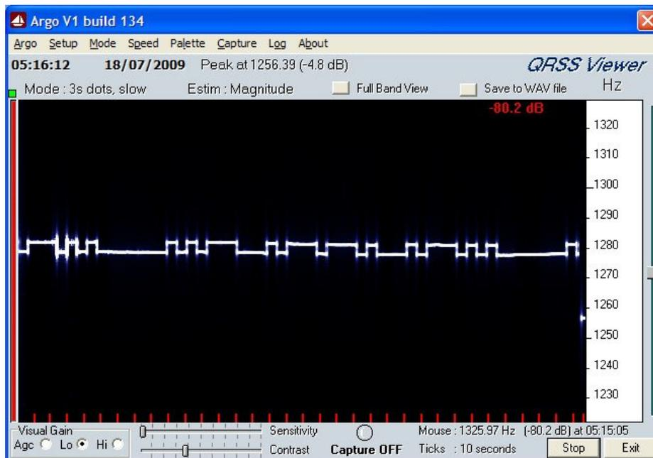
The “gimmick” capacitor C3 will need to be adjusted, to bring the “height” of the FSK to around 5Hz. Do not waste spectrum by using more! Twist C3 tighter to increase the shift, or unwind/snip some wire to decrease it.
