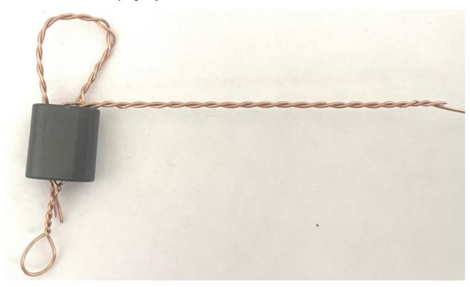
**Step 8:**Pull the twisted pair tight all the way through the binocular:
