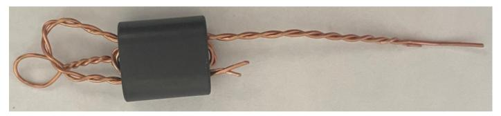
Slide the other twisted pair back through away from the twisted hairpin loop and pull both tight:
