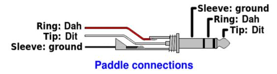
Don't worry if your paddle has a reversed pinout, or if you connect the dit and dah to a 3.5mm jack plug incorrectly: there is a configuration item in the configuration menu (CW Keyer menu) allowing you to swap the dit and dah in the firmware.
