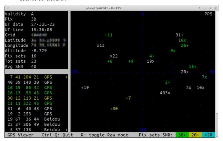
There is a + at the top right of the satellite list panel if you can use the up arrow to scroll up, and a + at the bottom right if you can use the down arrow to scroll down. The example shown here is a OLG2 with its standard active outdoor patch antenna and this is why you see very high SNRs, lots of satellites and both GPS and Beidou. The right-hand panel shows a sky map with all the satellites plotted on it.
