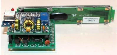
The Ultimate3 kit replaced the Ultimate2 less than a year later. The price of the attractive 16 x 2 blue backlit displays based on the HD44780 controller IC had come down so far that it wasn't much more expensive to upgrade to this nicer display instead of the surplus 24 x 1 LCD I'd used previously.
