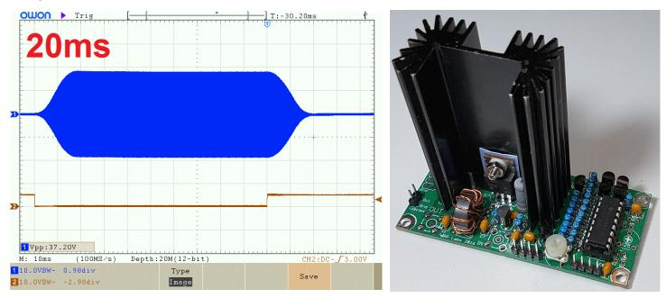
The circuit may be considered as a variable voltage regulator whose output voltage is set by a control voltage which may be provided from a Digital to Analog Converter (DAC) under microcontroller control. In our QMX case now, the chosen STM32 microcontroller has its own fast accurate internal 12-bit DACs so this is even easier.
