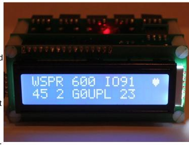
band weak signal modes QRSS/WSPR transmitter kit that provided a pile of functionality and fun.
