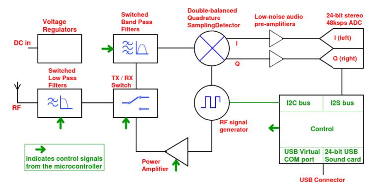
The receiver part of the design block diagram is a classic down-converting I-Q receiver, as used in many transceivers including the Elecraft KX2 and KX3. The performance of this receiver is determined largely by the dynamic range of the ADC and the noise floor (voltage input noise) of the op-amps used in the pre-amplifiers straight after the detector.
