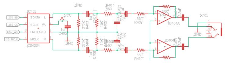
The audio output uses the same I2S 24-bit DAC chip, CS4334, as the QSX design. There are no accidents. The left and right channels separately drive two halves on an op-amp that drives the earphones. Keeping the channels separate will in future, allow things like gain adjustment to balance left and right channels for people with hearing defects, or in future, binaural reception.
