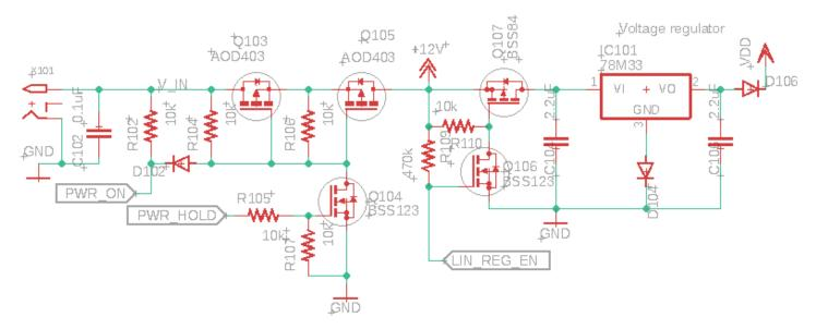
The solution is to include a 78M33 linear voltage regulator. At power up, the Q106 and Q107 switching circuits will ensure that the 78M33 linear voltage regulator is active. Then the
