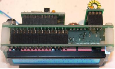
The Ultimate3S kit was a replacement for the Ultimate3, using an Si5351A chip designed onto a little daughterboard with a somewhat compatible pinout to the previous AD9850 DDS module so that it
