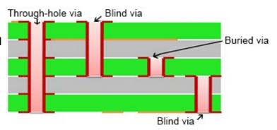
on the bottom side of the PCB under that location, for example – you can still connect a signal on the top layer of the PCB to an inside layer, by using a blind via. It doesn't go all the way though and contact with the SMD component on the bottom side. They're also useful when it comes to more groundplane stitching because again, you can do it underneath SMD components.
