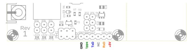
The 1pps, Serial data, TXD and RXD signals can be configured to be either 2.8V/3.3V logic level, or 5V logic level. The configuration is done using jumper wires that will be described in the next section. Note that 2.8V logic will be compatible with 3.3V systems, without issue.
