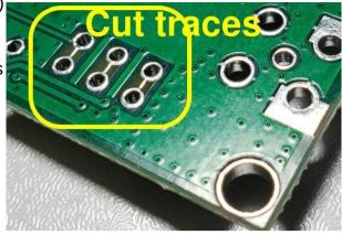
PCB, in order to disconnect the onboard LEDs. This should be done with a sharp knife, carefully so as not to damage any other nearby traces.
