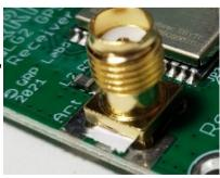
**Horizontal installation:** The SMA connector happens to fit the board nicely too in the horizontal, edge-mounted position. Place it with the center pin on the top side of the board, and two of the corner pins on the bottom side, and solder in place. The other two ground pins can be ignored. This works very well.
