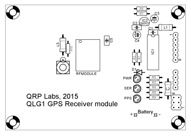
Pay special attention to the orientation of the semiconductor IC1. The dimple in the PCB silkscreen must be aligned with the dimple at the top of IC1.
