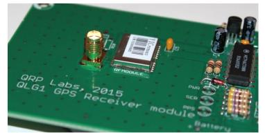
lower end of L3, to the SMA centre connector. This arrangement supplies power to the external antenna, from the RF Vcc supply output of the RF module. Note that it does not have short-circuit protection!
