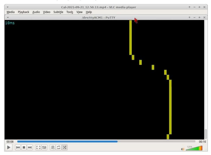
A fun and useful demonstration of the capabilities of QDX and the Input Analysis application, is to investigate the FT8 tone change transition. We know according to the WSJT-X documentation that to avoid splatter onto adjacent frequencies, WSJT-X makes a smooth transition between one tone symbol and the next. It's nice to be able to check this using the Input Analysis screen.
