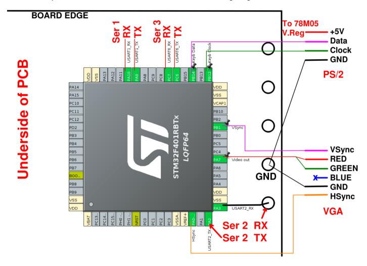
You may note that firmware 1 05 and above also have the possibility of a monochromatic VGA output and PS/2 keyboard connection. The VGA signal is generated directly on microcontroller
