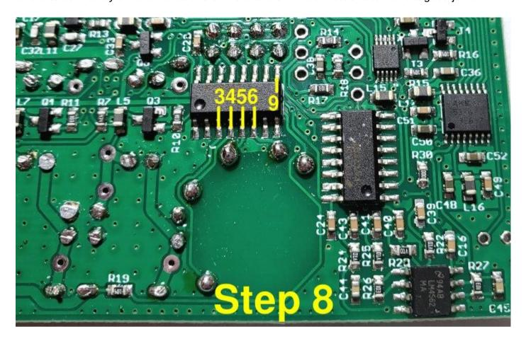
Here's the story so far, including the nicely installed L12 tapped inductor.
