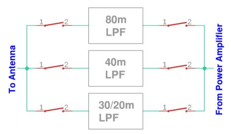
There is a PIN diode switch either side of each Low Pass Filter. So at any one moment, one pair of switches is activated, to switch the appropriate Low Pass Filter into the circuit.
