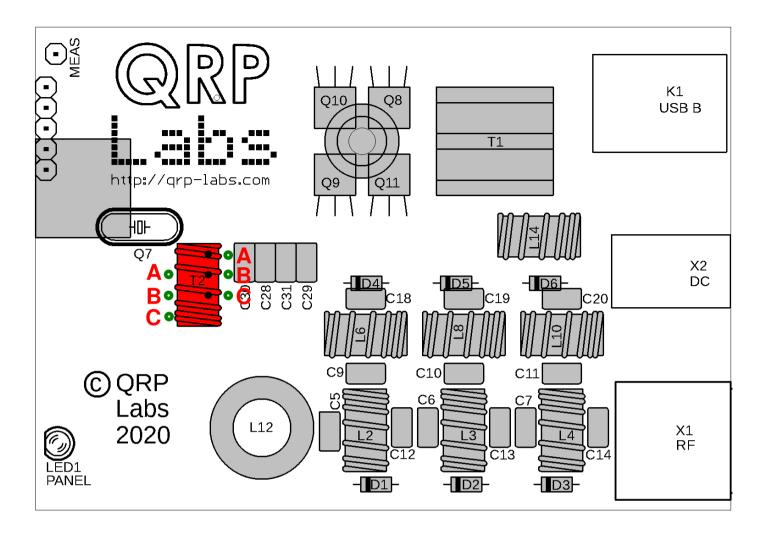
When you are satisfied that the wires are all in the correct holes, you can cut them to a length of about 2mm and solder them. It is best to cut-and-solder one wire at a time, since if you cut all the wires to 2mm length then the toroid is more likely to fall out before you've had a chance to solder any of the wires. If that happens, it will be tough to get all the wires back in the correct holes again.
