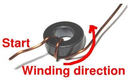
For all the toroidal inductors in the QDX kit, you will get it right, if you start as shown (photo, above right) and pass the wire through the toroid from the top side down through the hole, out and then around and over again; accumulating turns in the anticlockwise direction.
