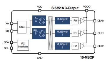
For best jitter performance, the Si5351A datasheet recommends the use of even integer dividers (no fractional component) in the MultiSynth dividers and in the QDX transceiver design, this recommendation is followed.
