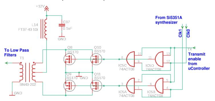
An interesting power amplifier circuit was designed specially for this transceiver. There are four BS170 transistors. Two are connected in parallel for the "push" side, and two connected in parallel for the "pull" side. Each side is driven by two AND gates of a 74ACT08 quad AND-gate IC, in parallel to ensure strong and fast drive.
