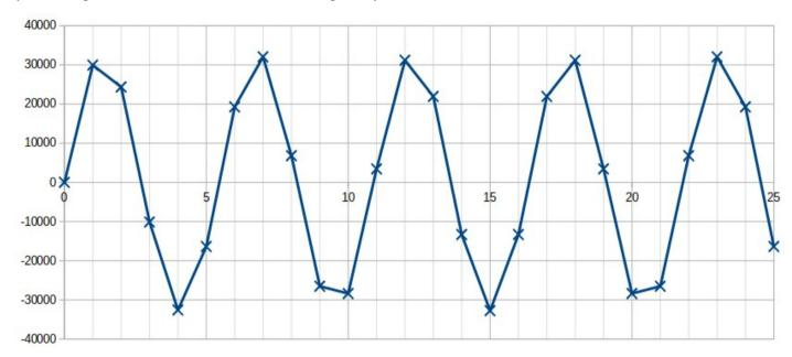
You can see that the sample points, indicated by the X's, are quite far apart. The zero-crossing time, or the time between the two samples adjacent to the zero-crossing, is a relatively large fraction of the cycle period. Our "x" is therefore not so small as it was before. The straight lines that previously didn't look at all bad, now look a lot less like the sinewaves that are being approximated.
