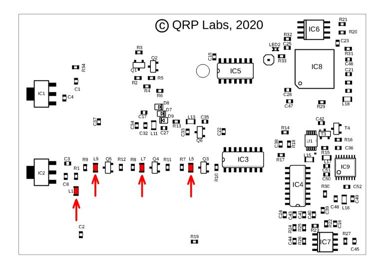
The diagram on the following page shows the best place to connect the leaded through-hole axial 47uH inductors. Do NOT try to connect the inductor leads to the tiny pads where the SMD inductors were installed – the pads are too delicate and will be ripped off too easily. Instead, solder them to a through-hole pad or a lead of an existing through-hole component.
