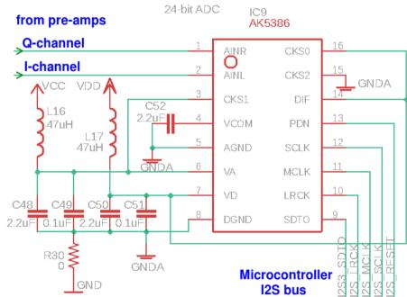
zero-ohm resistor R30 is the single point interface between the two grounds.
