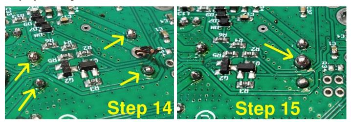
**Step 16**: Check that none of the wires protrude more than 2mm from the surface of the PCB, since if you are using the optional aluminium enclosure, there are only a few mm clearance.
