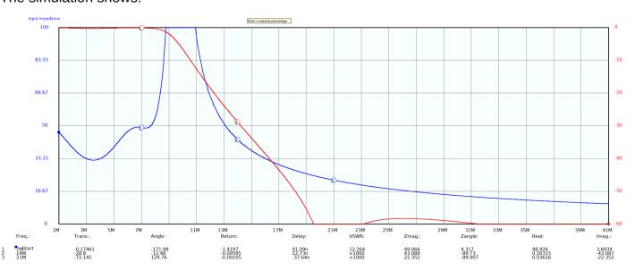
Fundamental: 7 MHz -0.17 dB Second harmonic: 14 MHz -28.8 dB Third harmonic: 21 MHz -72.1 dB
