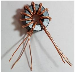
Now it's necessary to identify which wire belongs to which winding. You have three windings twisted together, they all use the same wire. The only way to do this is with a DMM as continuity tester. First, untwist and straighten the wire ends that are not wound around the toroidal core.
