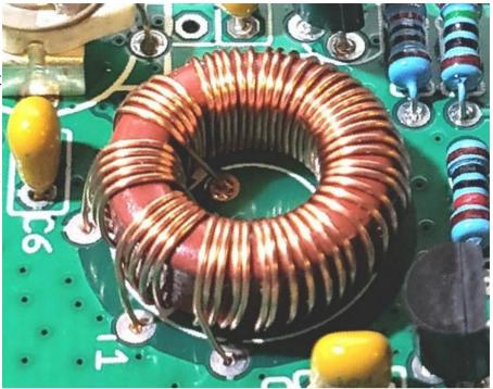
This transformer has FOUR windings. Three identical short windings, and one long winding. There are therefore eight wire ends, which must all be soldered into the correct holes on the PCB, and with the enamel properly removed.
