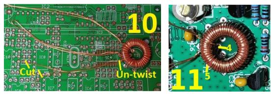
12) Next cut the 2<sup>nd</sup> loop, and un-twist the twisted section near the toroid body.
