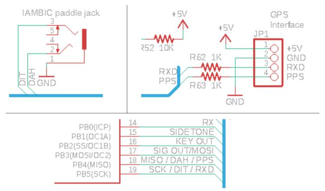
Secondly, consider the three different sections of the circuit diagram, shown above. It will be apparent that the paddle "Dit" signal is connected to pin 19 of the microcontroller, which is also the
