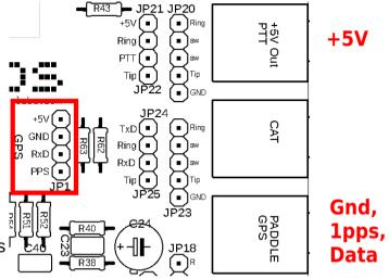
The GPS produces two output signals, PPS (Pulse-per-second) and RxD (Serial data), in addition to ground. Optionally +5V may also be connected, in order to power the GPS module. A GPS such as the QRP Labs QLG1 is perfect for this see <a href="http://qrp-labs.com/qlg1">http://qrp-labs.com/qlg1</a>
