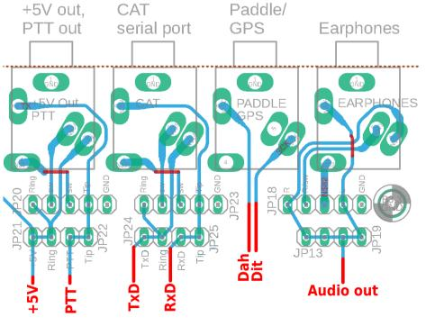
simple audio amplifier with a small loudspeaker. Installing two pins (one for audio, one for ground) and a corresponding socket on the underside of the QCX+ Dev board, would allow you to carry audio to the input of your audio amplifier from the tip "switch" pin of the 3.5mm socket, only when no earphones are plugged into the socket. In this way, you can arrange for your internal loudspeaker to automatically be used only when no earphones are plugged in.
