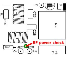
to pin 2 of the 4-pin DVM/RF Power header, then key-down, the display will read the power output in Watts. It is easiest to have the transceiver in Straight key mode and squeeze the paddle.
