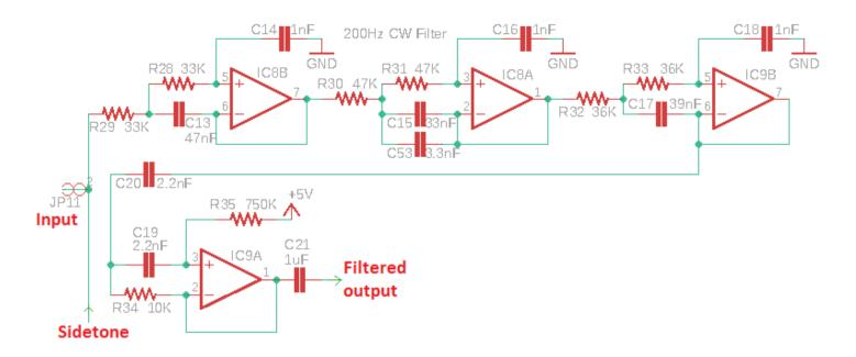
There are three stages of low-pass filtering and one stage of high-pass filtering. The first three stages retain the 2.5V "midrail" bias all the way through from the input transformer T1. The final stage IC9A is biased using the 5V supply (avoiding a few extra components to create a real 6V mid-rail at half the supply).
