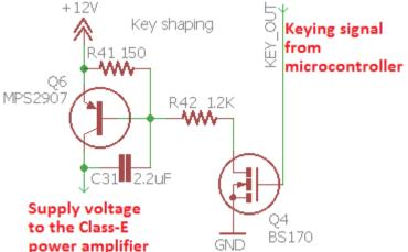
replaced by a straight Morse key to ground! But in our case, the microcontroller implements automated stored message sending, beacon modes, and lambic keyer – so we need the microcontroller to be the boss of everything. The microcontroller reads the state of the straight key or paddle, and processes it to produce a key output. When in straight key mode the
