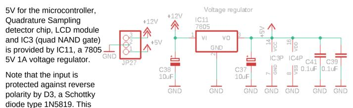
also drops the voltage by 0.3 to 0.4V, which has the effect of reducing the output power. D3 is shown on the microcontroller section of the circuit diagram, see earlier.
