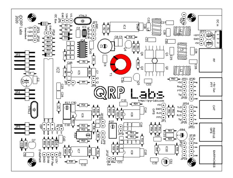
The number of turns in each winding depends on the band you are building the kit for. Refer to the following table. For convenience, the remainder of the instructions in this section refer to the 40m version (38 + 5 + 5 + 5 turns).
