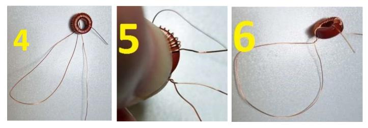
7) Do the same thing for two more loops, which are between the 43<sup>rd</sup> and 44<sup>th</sup> turns, and 48<sup>th</sup> and 49<sup>th</sup> turns respectively. It is easy to lose count. An easy way is after step 6, pass the wire through the hole 5 more times, and on the 5<sup>th</sup> one, make a loop. Similarly count
