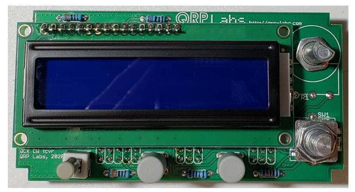
This photograph shows what the front panel PCB will look like, viewed from the rear. Notice the gain potentiometer, contrast trimmer, and pin header sockets are all on the rear side of the PCB.
