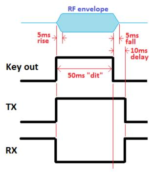
The Transmit/Receive switch must remain in "transmit" state for a short time after key-up, in order for the RF envelope of the key-shaping circuit to drop gently down to zero, which takes approximately 5ms. Due to this, the microcontroller implements a 10ms delay between key-up and switching the radio back to receive mode.
