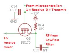
The transmit/receive switch is implemented by a single BS170 MOSFET. The source is at DC ground (via the primary of input transformer T1). The control signal from the microcontroller switches the MOSFET on or off. Interestingly, capacitor C34 close to the MOSFET gate is found to be necessary to prevent inductive pickup of the 5W RF from partially switching on the MOSFET.
