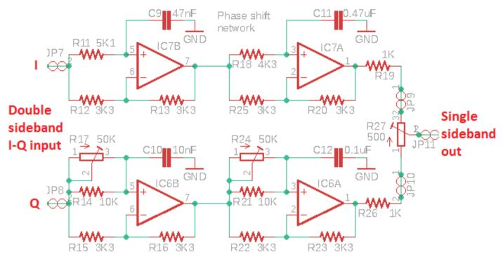
To improve the accuracy of the 90-degree phase shift, R17 and R24 allow adjustment of the phase shift at higher and lower audio frequencies respectively.
