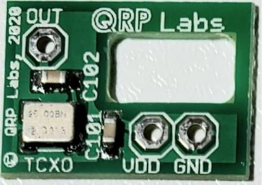
main QCX+ PCB. Note that the TCXO module is a 0.8mm thick PCB and is single-sided. The pads are quite delicate and it will not tolerate being de-soldered and re-soldered. In other words you need to be very careful to get this right the first time.
