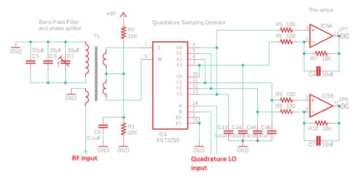
Since the band-pass filter, Phase splitter, Quadrature Sampling Detector and pre-amp circuits are so tied up together, I am going to consider them all together in this section.
