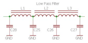
It is a 7-element filter design originally by Ed
