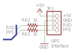
The optional GPS interface is provided by a 4-pin header at the bottom right of the board, next to the 3.5mm socket for the keyer. The pinout of the 4-pin header exactly matches the one on the QRP Labs Ultimate3S QRSS/WSPR transmitter kit, and the QRP Labs QLG1 GPS receiver kit. This makes connecting the radio to the QLG1 GPS kit very easy, if you wish. However other GPS modules could also be used. The following requirements of the GPS module must be met:
