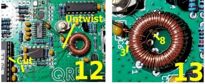
13) Similar to step 11; the wire which came over the toroid body has five turns then goes into hole 4, which you did in step 11. Insert this wire-end into hole 3.
