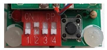
Start-up switch positions for serial port configuration
