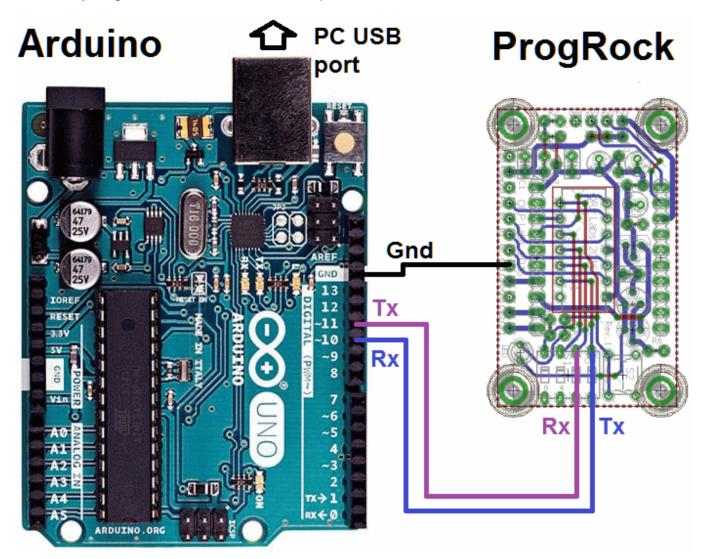
This short example sketch uses the Arduino SoftwareSerial library. Both ports are run at 9,600 baud. Received serial data on either input is re-transmitted to the other output.
