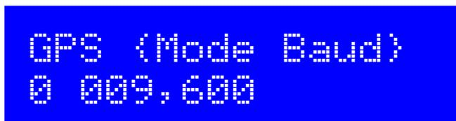
The first setting is the GPS mode. This controls how and whether GPS is used. If set to a non-zero value, and a GPS module is connected and producing a valid 1pps signal, then the accurate time pulses from the GPS unit will be used to keep precise time. In the event of a GPS signal outage (for example, poor reception), the kit will continue to use the on-board 20MHz crystal oscillator for time-keeping.
