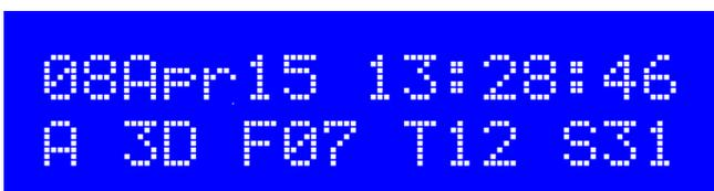
The display shows date and time on the top line, followed by GPS satellite reception information on the bottom line. The heartbeat will blink in the space between the date and time on the top line.
