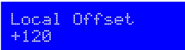
This setting specifies the offset of local time to UT. The time displayed by the #HH, #MM tags is always UT (straight from the GPS, if connected). The #LH, #LM, #AP and #H2 tags display local time, offset by the number of minutes in this setting. Additionally, Local date tags are available, these are #ND, #NM and #NY representing day, month and year respectively.
