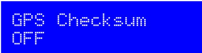
This Boolean setting controls whether the checksum validation is performed on the GPS data NMEA sentences. If set to ON, and the checksum validation fails (for example due to noise corrupting the data on the wires), then the invalid data is ignored.
