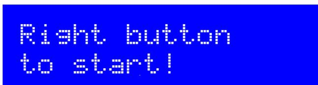
Finally, at the end of scrolling through all the configuration menu items, this screen is displayed. Now simply press the Right button, to start the kit in its display sequence.
