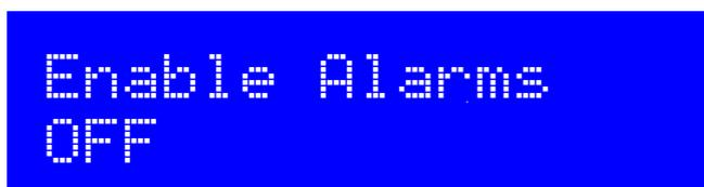
This Boolean parameter comes after the 10 alarms. **It enables or disables all ten alarms together.** It is a global enable override for the alarm system. In order for a particular alarm to be activated, the following three conditions must all be met:
