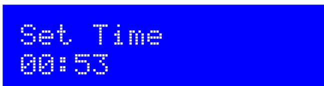
This setting is only required if you have NOT connected a GPS receiver module to the kit. If a GPS is connected, the time should be set automatically.
