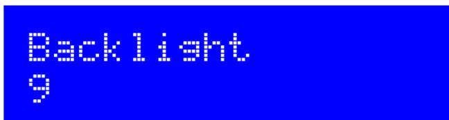
This setting allows the LCD screen's blue LED backlight brightness to be adjusted. The default value is 9 (maximum brightness). 0 corresponds to minimum brightness – the backlight is switched off.
