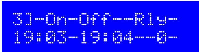
To edit the other fields of the alarm configuration, scroll through the menu using the left button, to find the desired alarm. Press the right button ONCE to begin editing. The top left corner character begins to flash. Now press the left button again, to move the cursor to the 10's of hours digit of the alarm ON time. The alarm ON time is the time at the bottom left.
