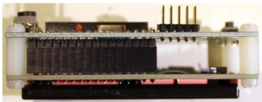
perfect alignment. Use the eight 6mm M3 screws, and four 12mm nylon hex spacers, to bolt the PCB to the LCD.
