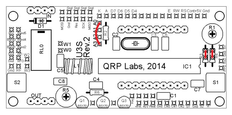
**Optional resistor R3**: This can be fitted to enable in-circuit-programming for those wishing to update their own firmware (and having the necessary equipment). Use a 100K resistor to pull IC1's "reset" input high, so that the in-circuit programmer can control the signal during programming.
