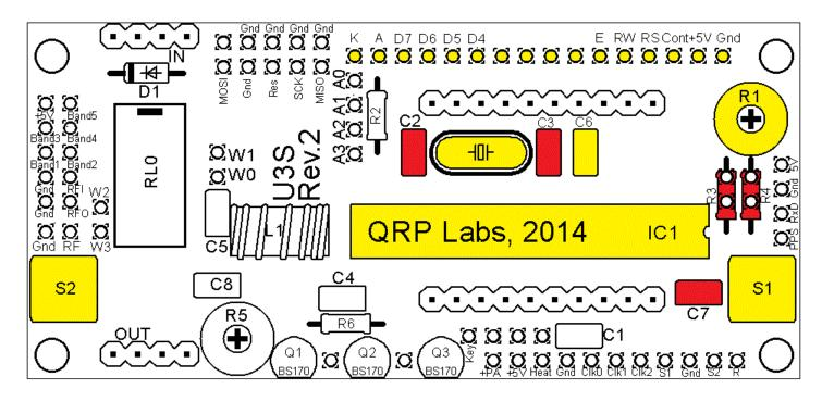
Pay special attention to the orientation of the semiconductor IC1. The dimple in the PCB silkscreen must be aligned with the dimple at the top of the IC socket and the IC.
