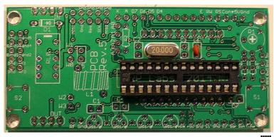
I recommend NOT installing them. Some crystals do not oscillate reliably with 22pF capacitors, but apparently they will work fine without any capacitors; the board and lead parasitic capacitances are sufficient for reliably operation. It does not matter that the oscillation frequency will not be exactly 20MHz, this is compensated in software.
