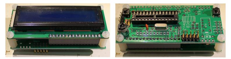
Important! Upon power-up, you will need to adjust the contrast potentiometer R1 to view the LCD properly. Turn it fully clockwise to start with (before applying power). Then turn it gradually anticlockwise until the displayed text looks correct.
