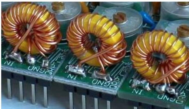
**Do not solder the “hot” (non-ground) end of the main toroid windings yet! This will be done temporarily first before installation in the PCB hole – see “Adjustment” step, below.**
