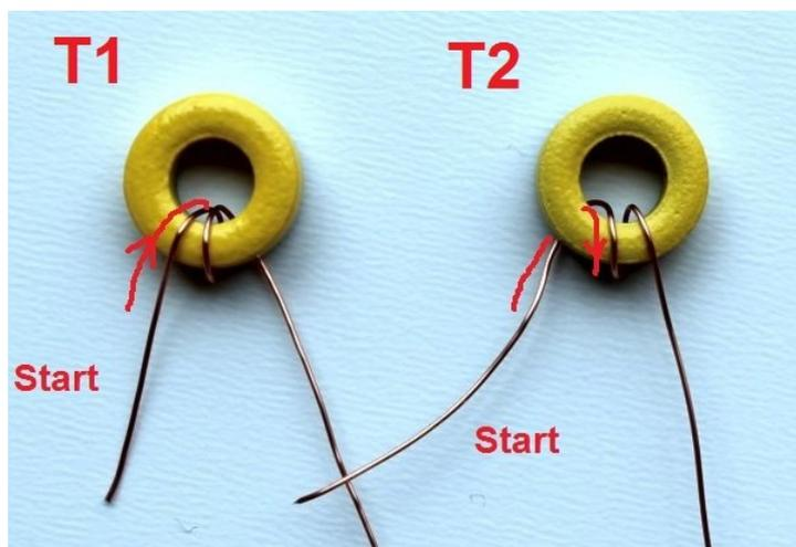
It should be clear that for the left toroid, the wire passes over the top of the toroid and through the hole, to start with. But for the toroid on the right, the wire passes behind the toroid and through the hole, towards us.
