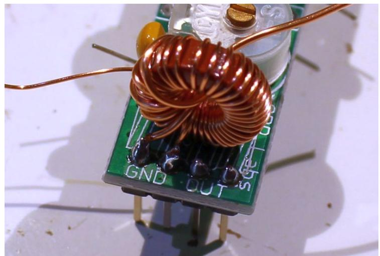
wire end in a blob of molten solder for some seconds until you can see that the enamel is burnt away and the wire is tinned, ready for soldering.
