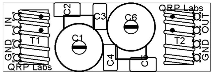
Temporarily solder the “hot” winding ends of T1 and T2 to the un-cut wires sticking out of C2 and C5
