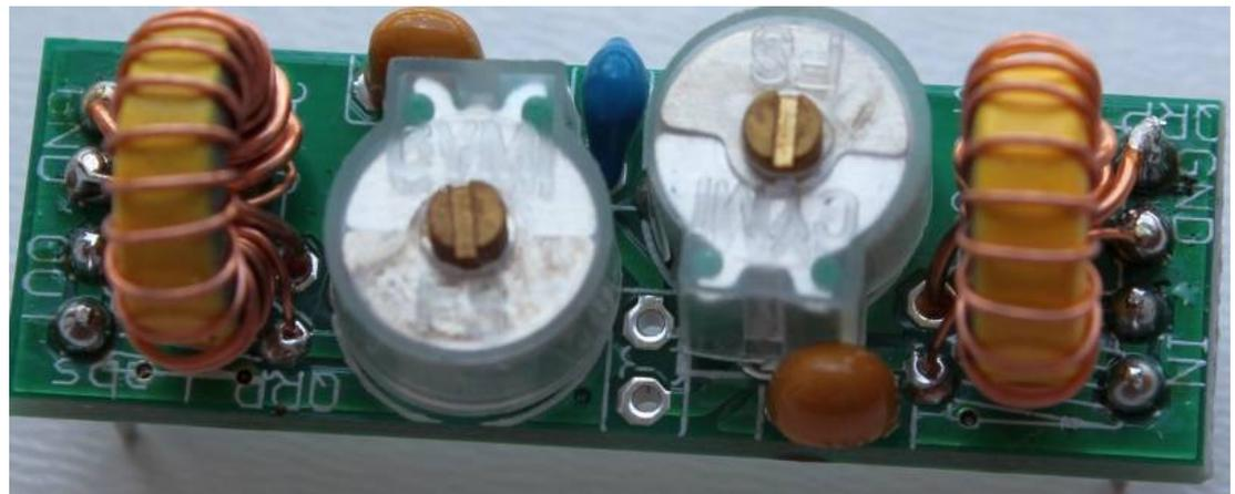
Maximum capacitance (“closed”). You can see that the plates of the trimmer capacitors overlap each other completely.
