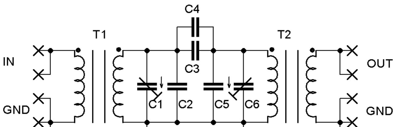
Please read and follow this assembly manual carefully, step by step. The band pass filters require careful construction and adjustment. Generally the adjustment is more difficult for the lower frequency bands.
