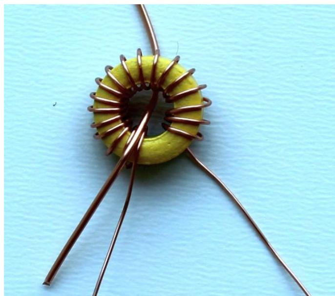
The photo (right) shows the completed second winding (thick wire). There are THREE turns in the 15m BPF. **Check the number of turns required, for the band you are building (see parts list).** Remember that each time the wire passes through the central hole of the toroid, counts as one turn.
