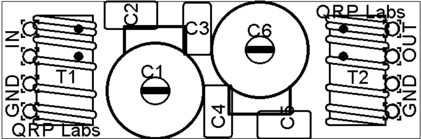
The PCB is quite small and the parts are close together. You are recommended to use a low wattage iron with a fine tip, and fine solder e.g. 1mm diameter or less. Take care not to overheat the PCB and risk damaging it. A well-lit area and magnifying glass may assist. Be careful not to bridge solder across closely-packed connections. I recommend checking with a DVM to make sure no solder bridges have been inadvertently created. Take care to ensure correct alignment of the 4-pin plugs.
