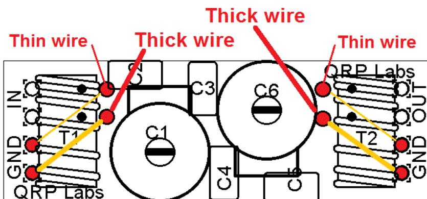
(for T2). The other ends of the toroidal transformer windings are both connected to ground pins (“GND”) so it does not matter which is the thin wire and which is the thick wire.
