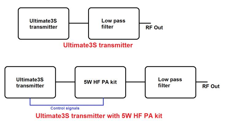
The basic Ultimate3S transmitter is shown in the top half of this diagram. The Low Pass Filter (the LPF) is drawn as a separate block to the Ultimate3S transmitter. In reality the LPF is a plug-in module on the Ultimate3S PCB. If you are running a multi-band Ultimate3S then there is a LPF plugged into your Ultimate3S PCB, and a 5-band Relay-switched extension PCB bolted behind that. As far as the 5W HF PA kit is concerned, the principles are the same in the single-band and multi-band cases.
