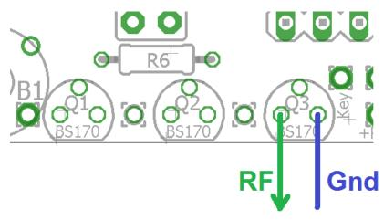
connected to the "RFI" pin of that 2 x 5 header such that everything lines up when the boards are stacked together. This applies whether you are using the single-band or multi-band system.
